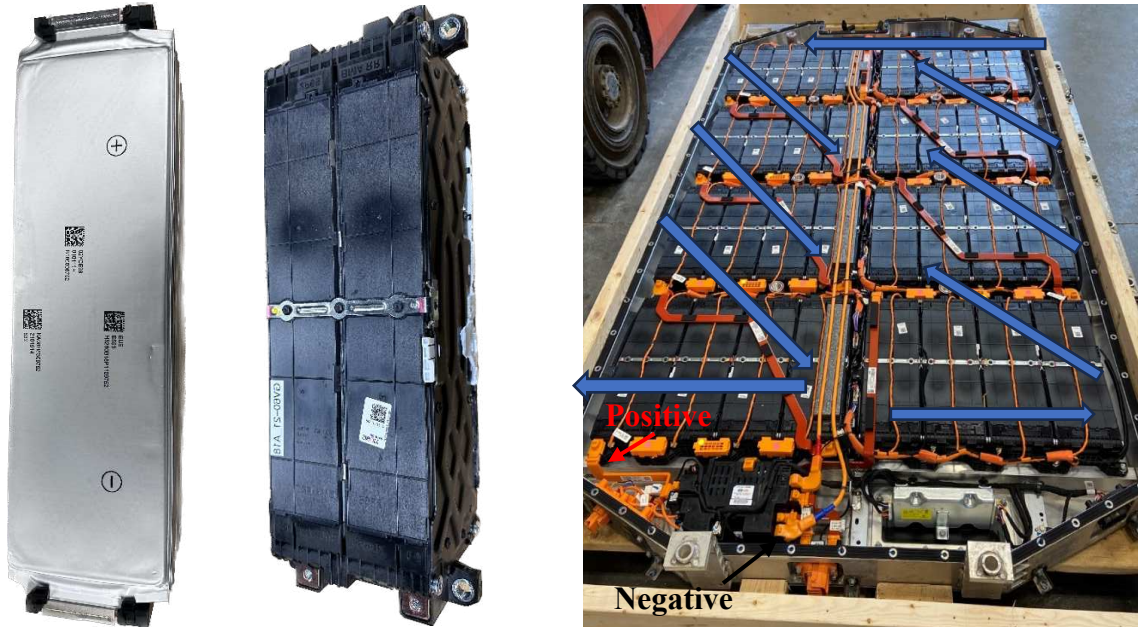
Figure 4.4: a) Genesis GV60 NMC cell (Left); b) GV60 Module (Middle); c) GV60 Pack (Right)
