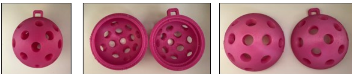
Figure S1. The COVID-19 Sewer Cage (COSCa), is a passive sampling device for monitoring SARS-CoV-2 in municipal wastewater.
