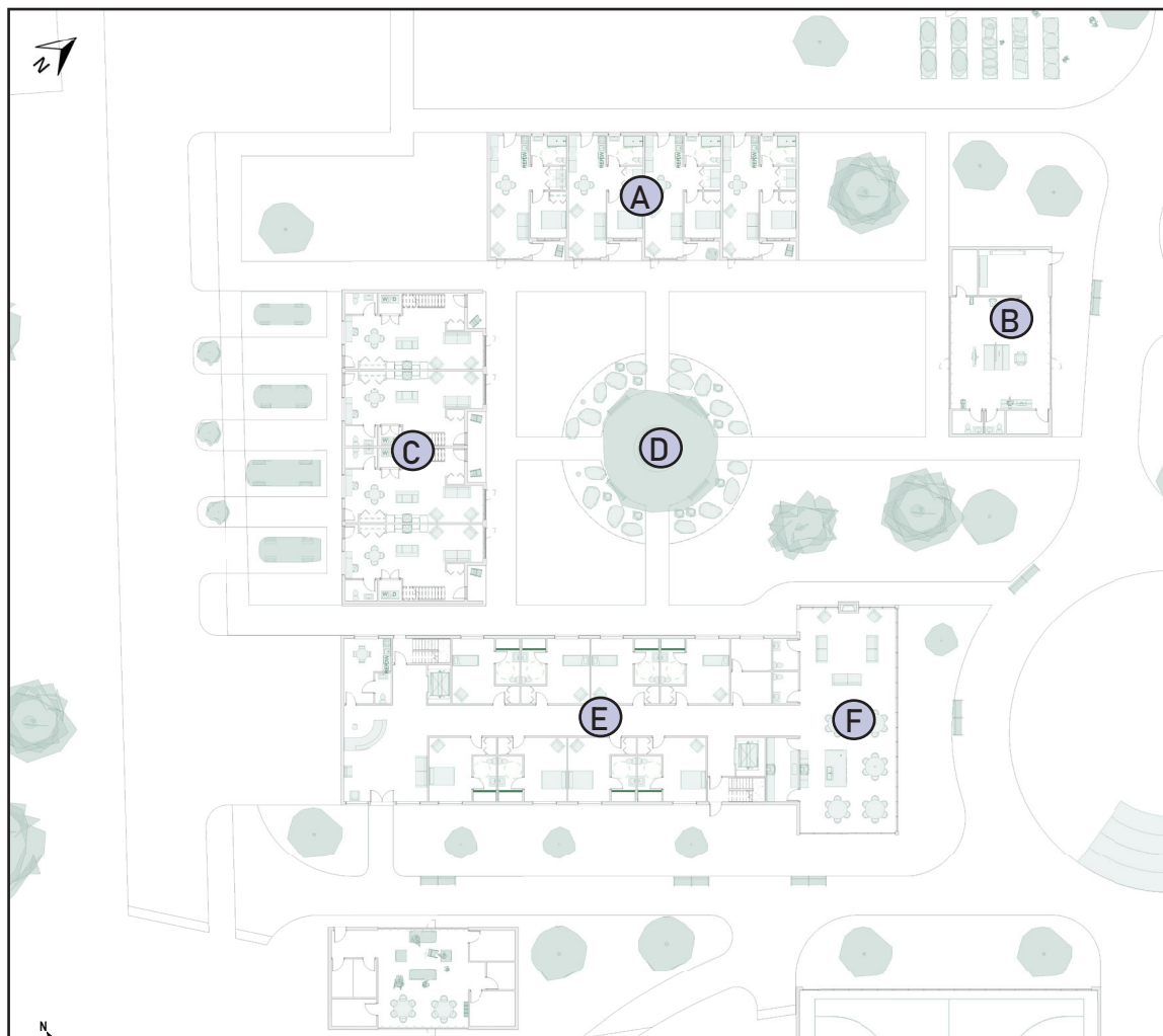
Neighbourhood 1 Ground Floor Plan. A - Independent Living Rowhousing, B - Workshop, C - Family Rowhousing, D - Shared Courtyard, E - Assisted Living, F - Shared Dining and Living Space.
