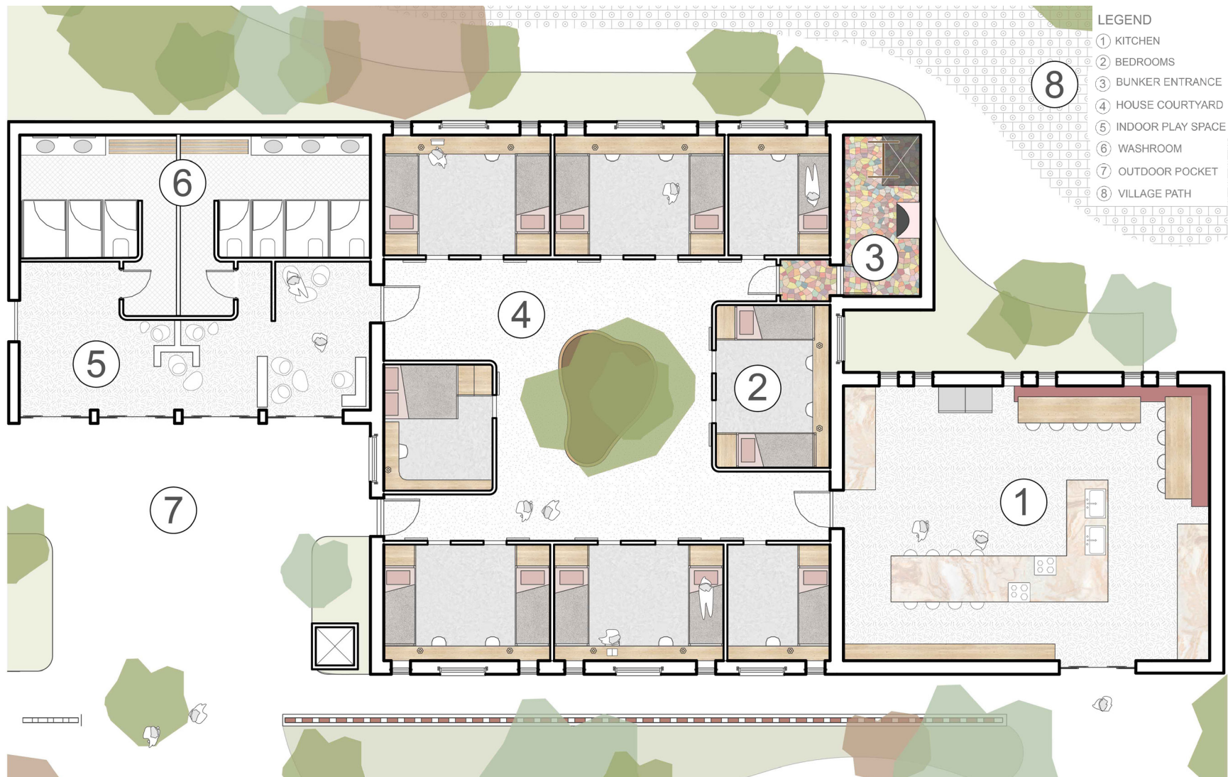
Figure 65: This floor plan is a single house plan with a shared kitchen on the right and shared washrooms/changing rooms on the left.
