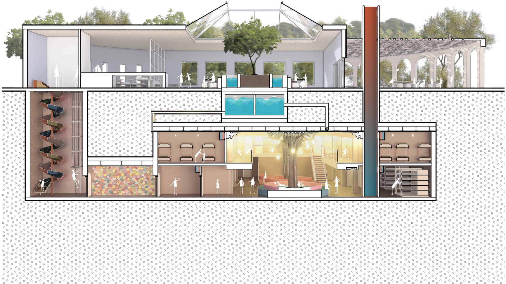
Figure 71: This section is taken within the Majless connecting to the bunker down below. It displays the hidden water source, wind tower, and ventilation that is provided for the bunker space. It also displays the relationship of the bunker's play areas with the sleeping areas located on the mezzanine. To the left of the section, there is one of the four entrances/exits to the bunker that holds a slide for accessibility and a step ladder.
