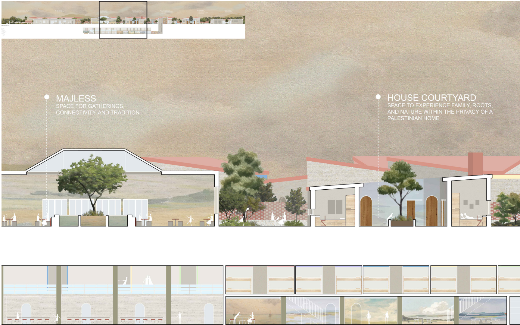
Figure 87: In the third/middle part of the major section, we have the Majless as well as the bedrooms and courtyard of a single house cut through.
