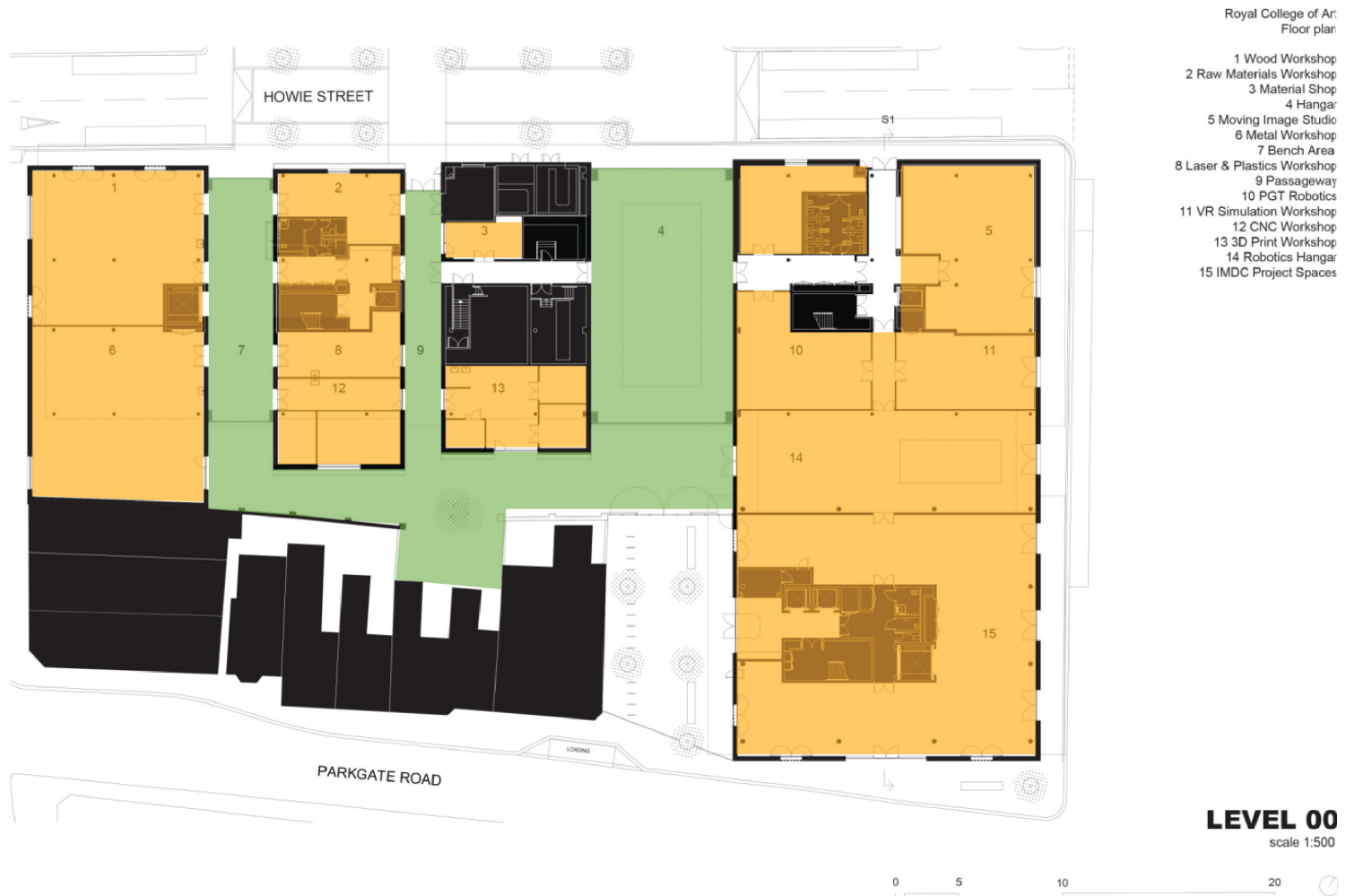
Diagram analysis of the ground floor programmatic layout relationship between interior programmes (orange) with outdoor spaces (green). Herzog & de Meuron, plan of Royal College of Art, London, 2021 (Herzog & de Meuron 2021).
