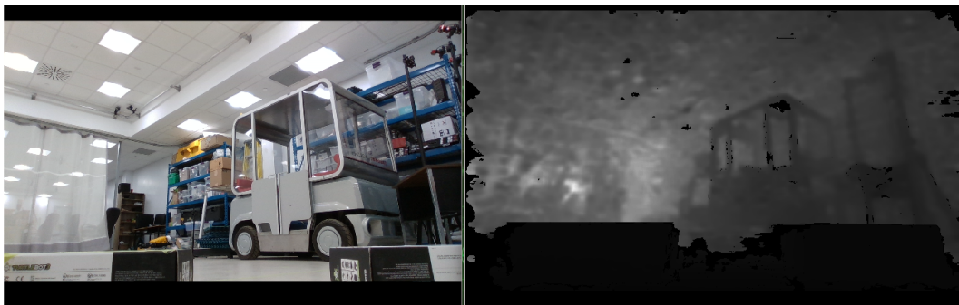
Figure 5.5. Leader depth camera view during narrow gap passing, RGB(left), depth(right)
