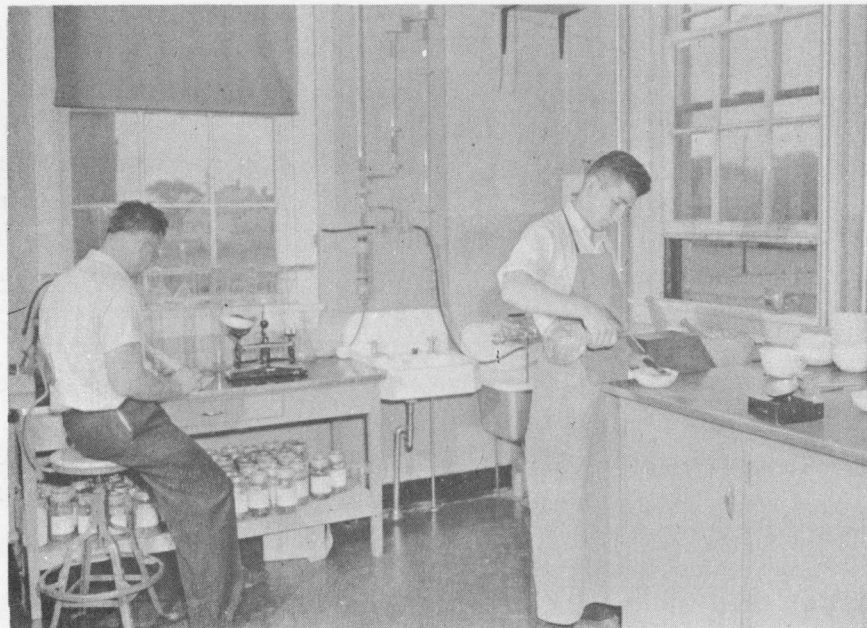
Fig. 16 - A view of the soil mechanics laboratory where pre-investigation of fill and foundation conditions is carried out from samples obtained in the field.
