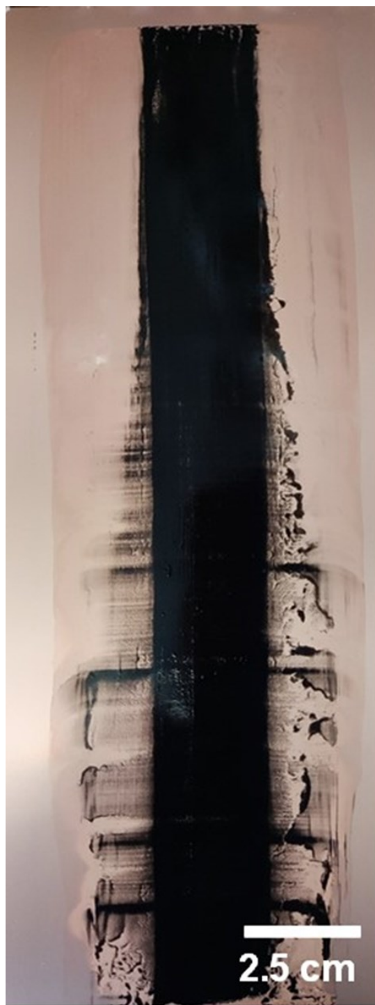
Figure 3.3 A picture of the coating made from SiO from a water-based slurry with 1.2k NaPAA.
