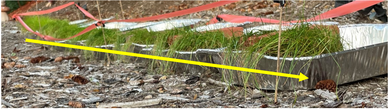
Figure 48 - Outdoor hydroseed trial 1 - 6 weeks post plant. Yellow arrow denotes direction of increasing sludge percentage. Growth containing Kentucky Bluegrass ( Poa pratensis ), Creeping Red Fescue ( Festuca rubra ), Perennial and Annual Ryegrass ( Lolium perenne and Lolium multiflorum ). Treatments of 0-100% sludge were utilized.
