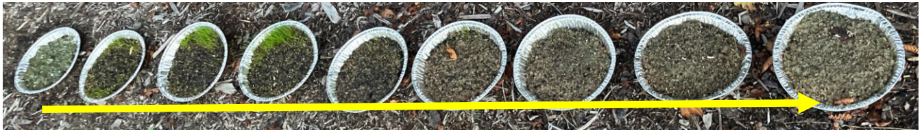
Figure 54 - Outdoor hydroseeded trial 2 - 1 week post plant. Yellow arrow denotes direction of increasing sludge percentage. Growth containing Kentucky Bluegrass ( Poa pratensis ), Creeping Red Fescue ( Festuca rubra ), Perennial and Annual Ryegrass ( Lolium perenne and Lolium multiflorum ). Treatments of 0-100% sludge were utilized.
