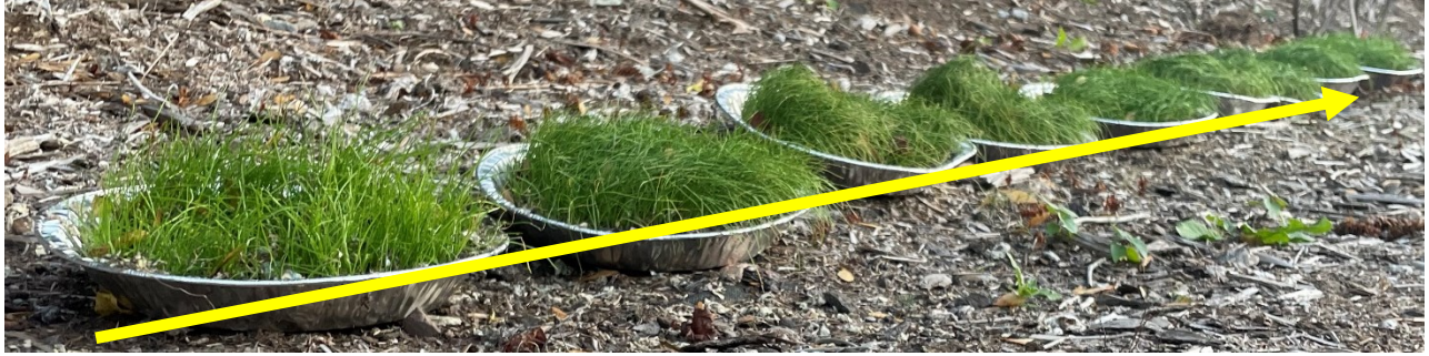
Figure 55 - Outdoor hydroseed trial 2 - 2 weeks post plant. Yellow arrow denotes direction of increasing sludge percentage. Growth containing Kentucky Bluegrass ( Poa pratensis ), Creeping Red Fescue ( Festuca rubra ), Perennial and Annual Ryegrass ( Lolium perenne and Lolium multiflorum ). Treatments of 0-100% sludge were utilized.
