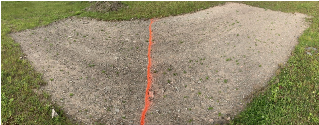
Figure 36 - Initial 15 x 7' laydown area for hydroseed trials. The left side represents the use of Celumulch and the right side represents the use of sludge.
