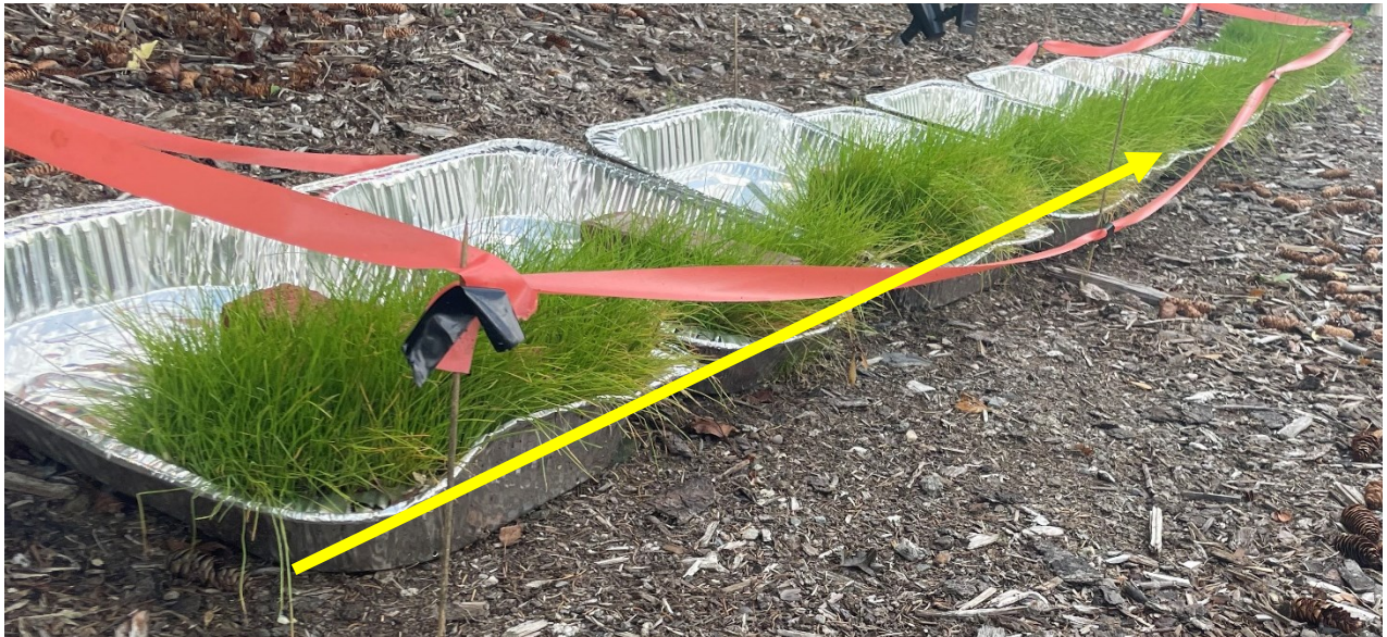
Figure 47 - Outdoor hydroseed trial 1 - 5 weeks post plant. Yellow arrow denotes direction of increasing sludge percentage. Growth containing Kentucky Bluegrass ( Poa pratensis ), Creeping Red Fescue ( Festuca rubra ), Perennial and Annual Ryegrass ( Lolium perenne and Lolium multiflorum ). Treatments of 0-100% sludge were utilized.
