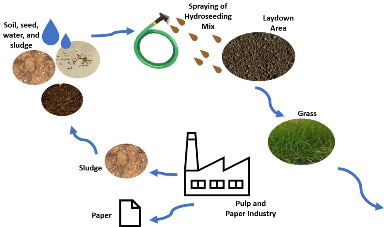
Figure 1 - General flow of materials utilized in sludge, from industry waste to final grass product.
