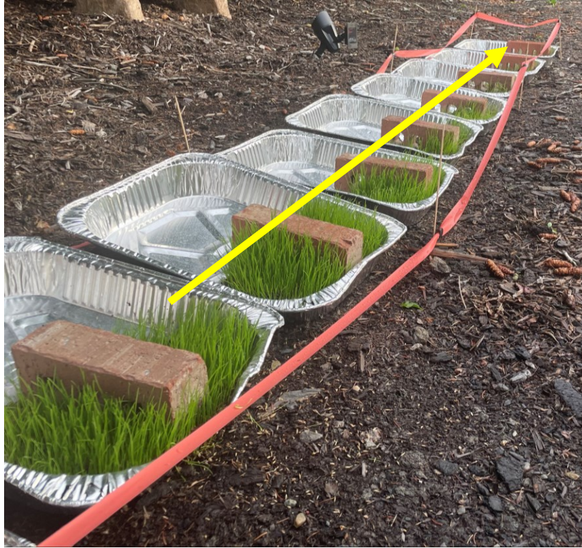
Figure 45 - Outdoor hydroseed trial 1 - 1 week post plant. Yellow arrow denotes direction of increasing sludge percentage. Growth containing Kentucky Bluegrass ( Poa pratensis ), Creeping Red Fescue ( Festuca rubra ), Perennial and Annual Ryegrass ( Lolium perenne and Lolium multiflorum ). Treatments of 0-100% sludge were utilized.
