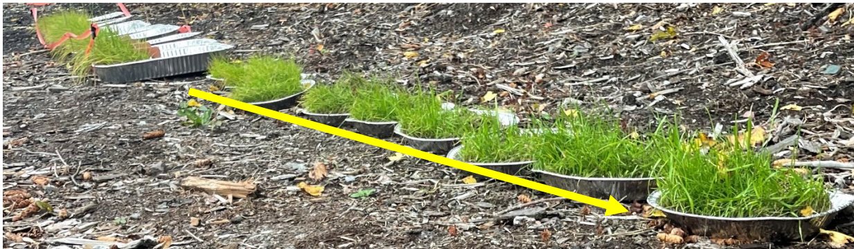
Figure 56 - Outdoor hydroseed trial 2 - 5 weeks post plant. Yellow arrow denotes direction of increasing sludge percentage. Growth containing Kentucky Bluegrass ( Poa pratensis ), Creeping Red Fescue ( Festuca rubra ), Perennial and Annual Ryegrass ( Lolium perenne and Lolium multiflorum ). Treatments of 0-100% sludge were utilized.
