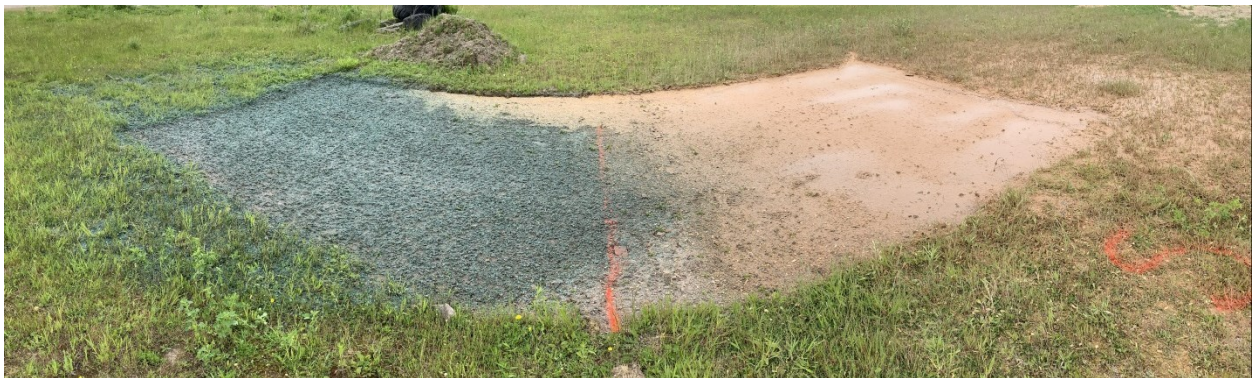
Figure 38 - Panoramic view of laydown area immediately following hydroseed application. Left-hand side represents typical hydroseed mixture and right-hand side represents sludge based hydroseed mixture. Sides contained grass growth composed of 40% Creeping Red Fescue ( Festuca rubra ), 30% Perennial Ryegrass ( Lolium perenne ), and 30% Kentucky Bluegrass ( Poa pratensis ).
