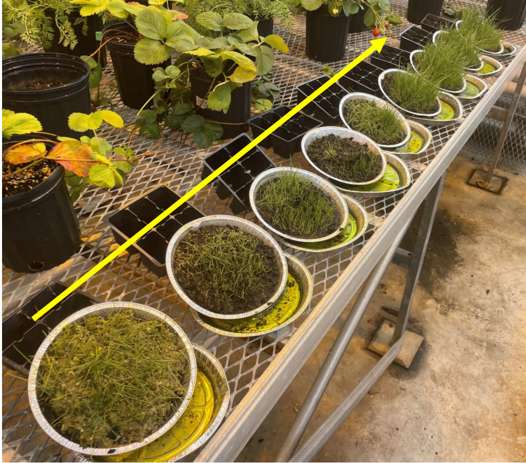
Figure 51 - Indoor hydroseeding trial 1 - 2 weeks post plant. Yellow arrow denotes direction of increasing sludge percentage. Growth containing Kentucky Bluegrass ( Poa pratensis ), Creeping Red Fescue ( Festuca rubra ), Perennial and Annual Ryegrass ( Lolium perenne and Lolium multiflorum ). Treatments of 0-100% sludge were utilized.
