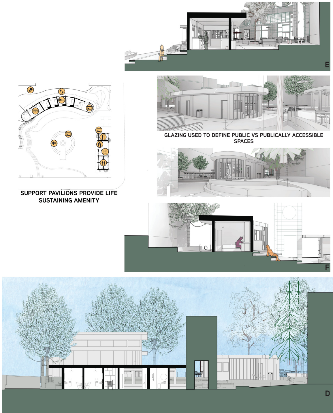
Fig. 32: “Supportive Space” these pavilions flank the two sides of the site and act as a threshold, in terms of the personal hygiene pavilion that anchors the Hamilton, Dunsmuir corner. Then the rest and rejuvenation pavilion creates a border to the site and sits privately up the terraced landscape.
