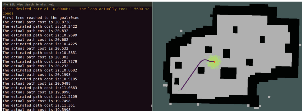
Figure 5.15: Test 3: Replan Twice and Bypass the Third Obstacle.
