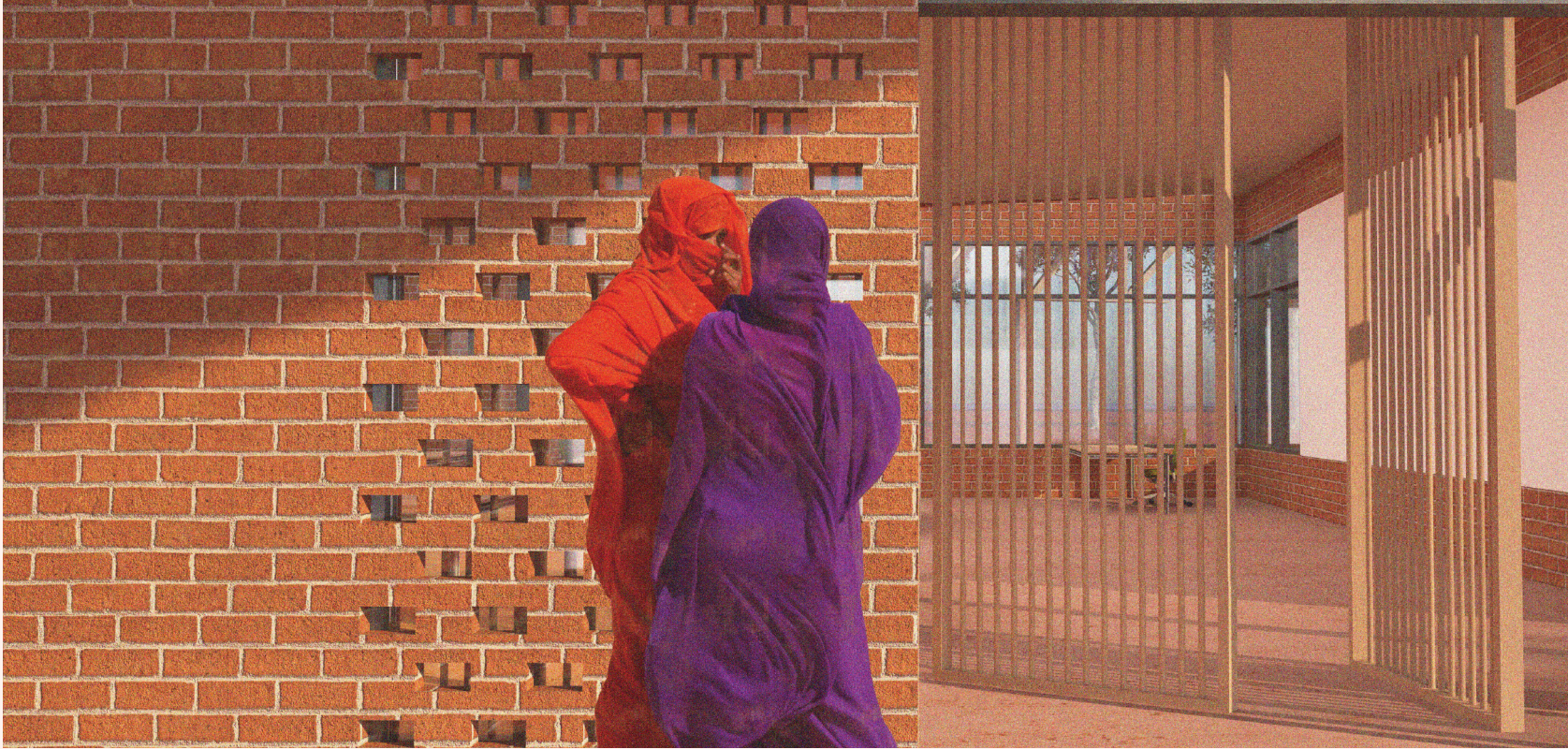
Elevation detail of brick wall becoming increasingly porous as it meets with key windows
