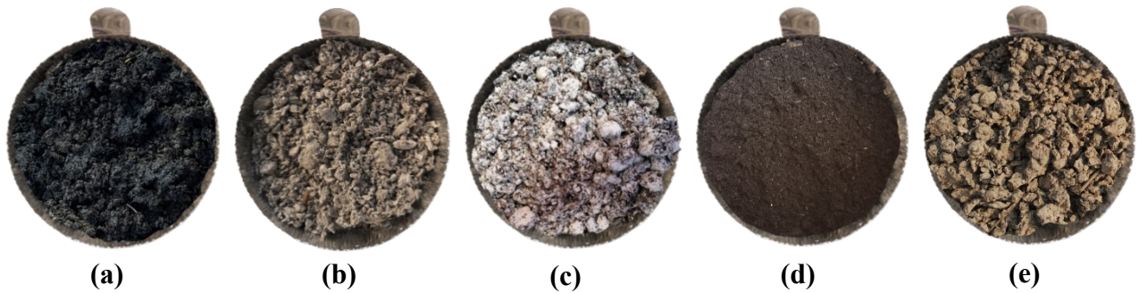
Figure 2. 1 Dewatered raw sewage sludge (a), N-Viro (b), CaO-treated (c), and composted (d), and heat-dried (e) biosolids.
