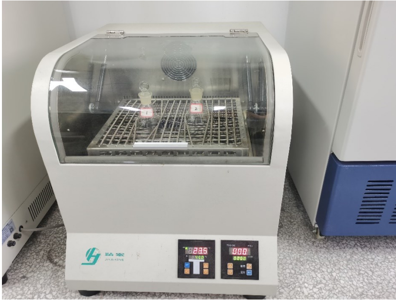
Figure S3.1 The temperature-controllable shaker.
