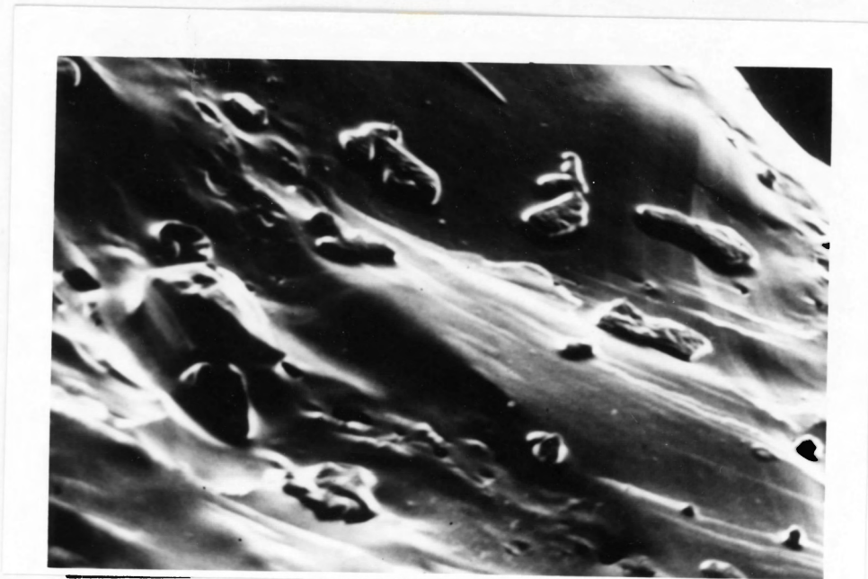
Angular quartz grain showing high relief and conchoidal fracturing.
