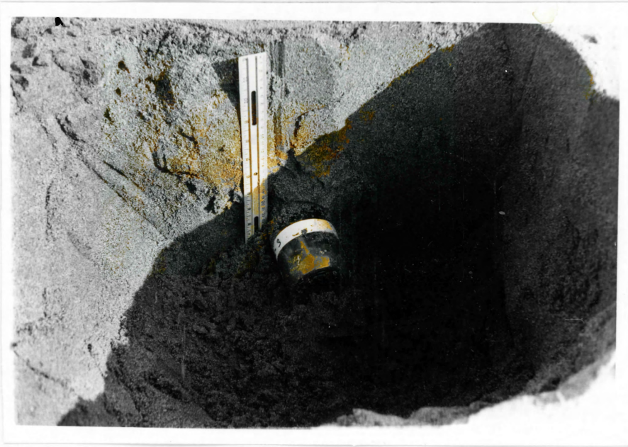
Plate 2: Beach Sample Collection Technique.
