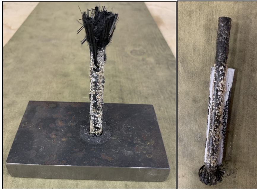
Figure 3-14. Pinching Shear CFRP Failure Mode
