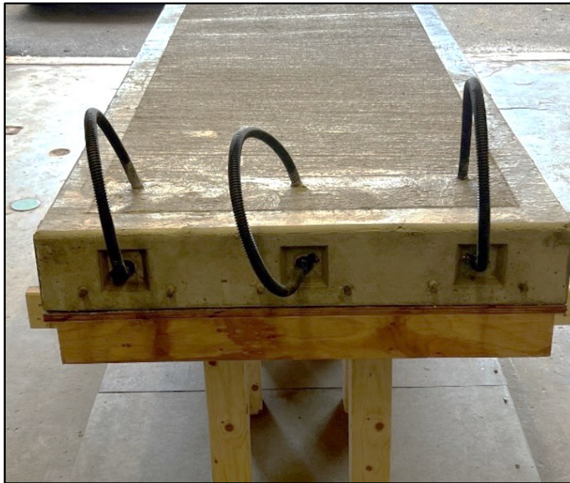
Figure 4-6. Control Specimen Jacking End
