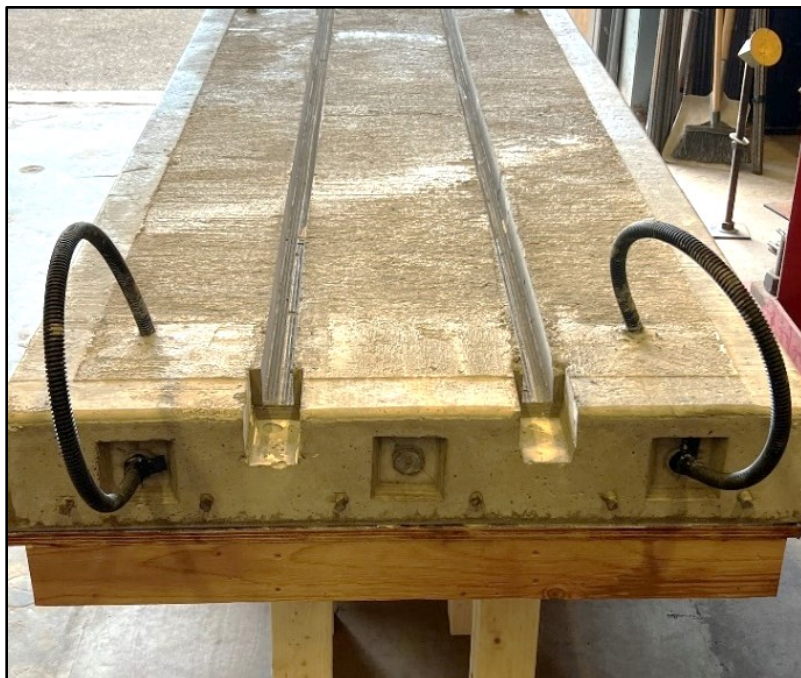
Figure 4-7. Rehabilitation Specimen Jacking End
