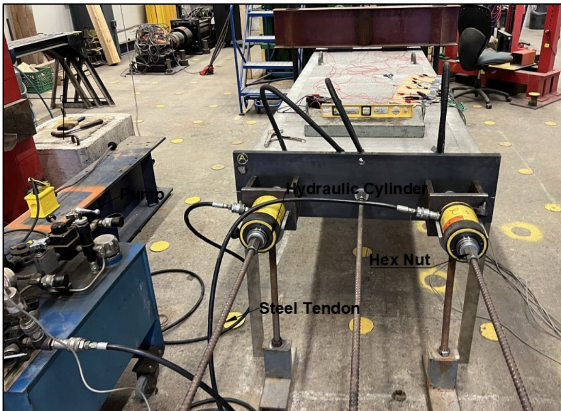
Figure 4-9. Control Specimen Post-Tensioning Operations
