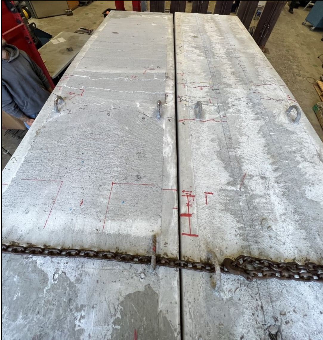
Figure 4-31. Bridge Cantilever Specimens Top Slab Side by Side Photo
