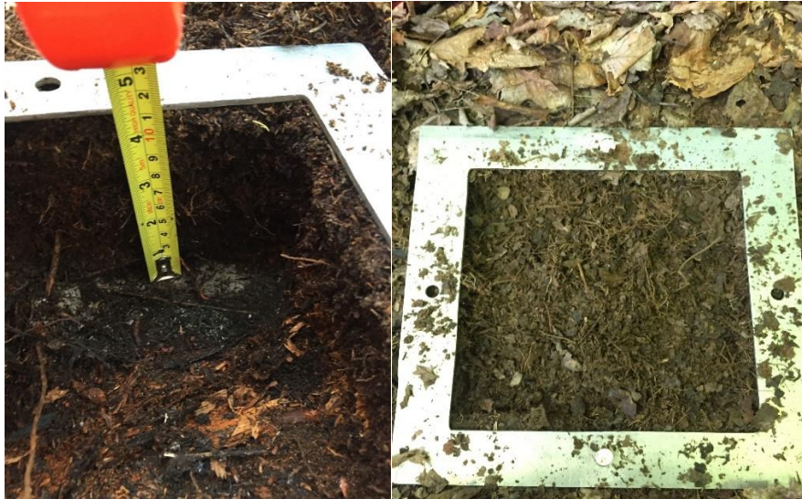
A4 Figure 5. Forest floor bulk density sampling at the Otter Ponds Demonstration Forest softwood (left) and hardwood (right) sites using a 20 cm X 20 cm metal square in which all forest floor within the square up to the mineral soil was sampled.
