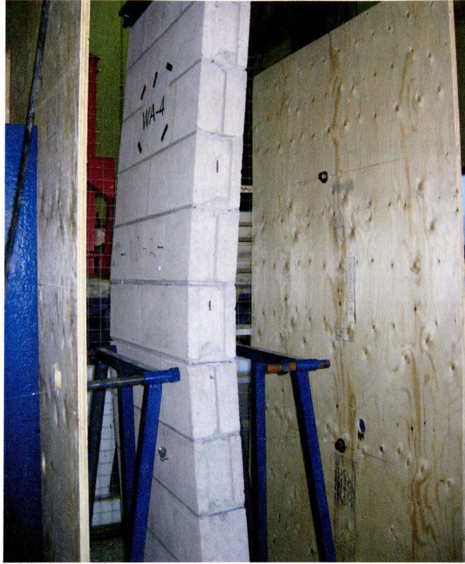
Figure 4.4 Failure mode of wall specimen WA-4
