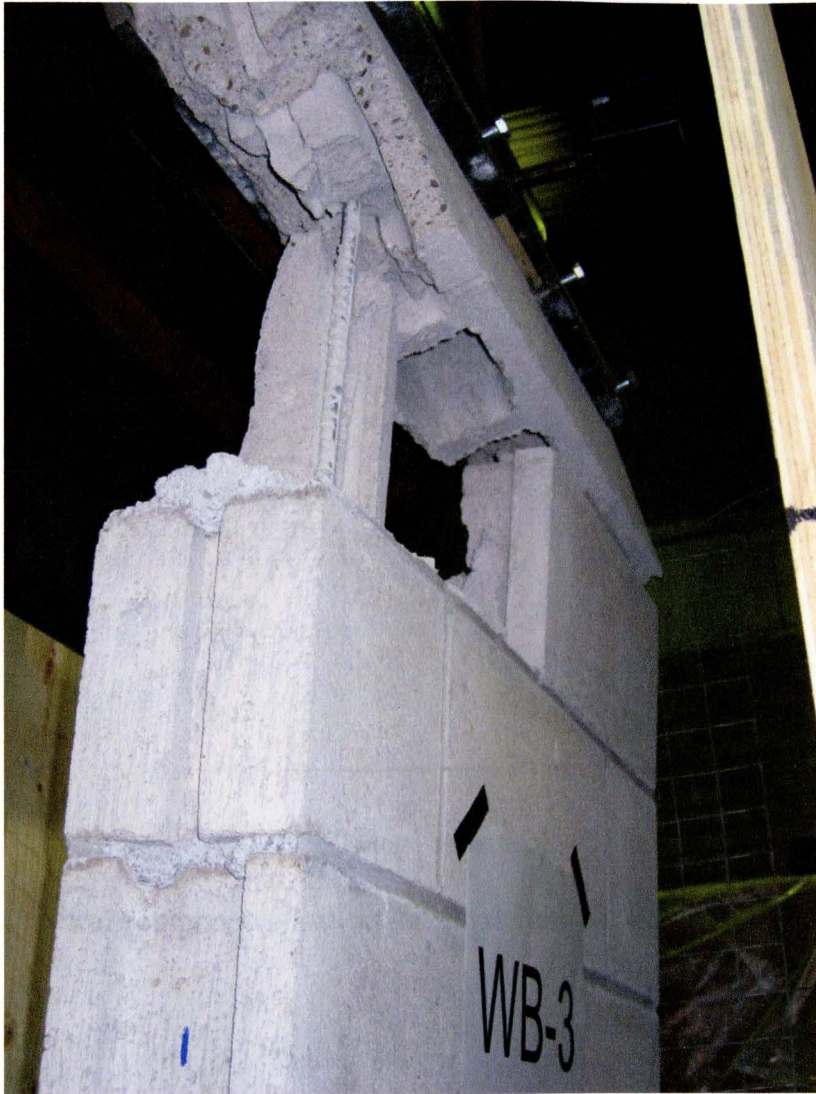
Figure 4.12 Failure mode of wall specimen WB-3
