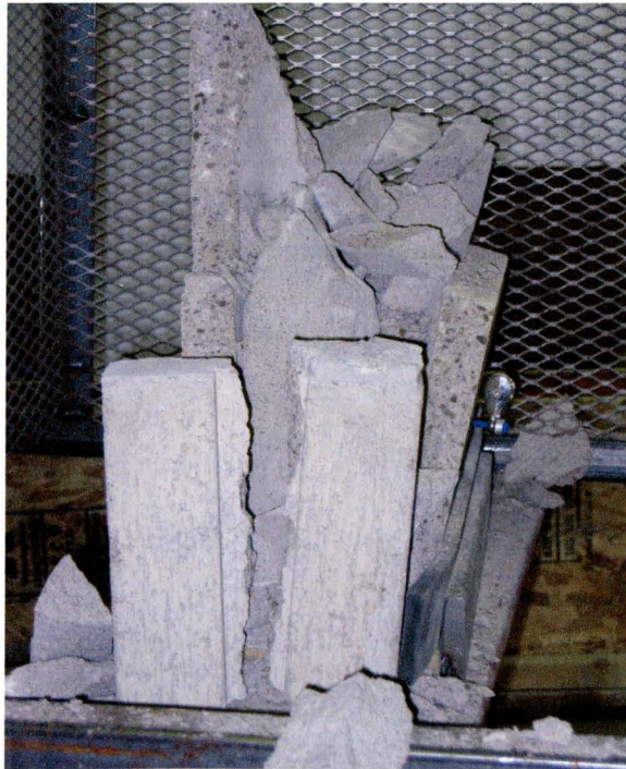
Figure 3.19 Failure mode of 3-high fully grouted prism test
