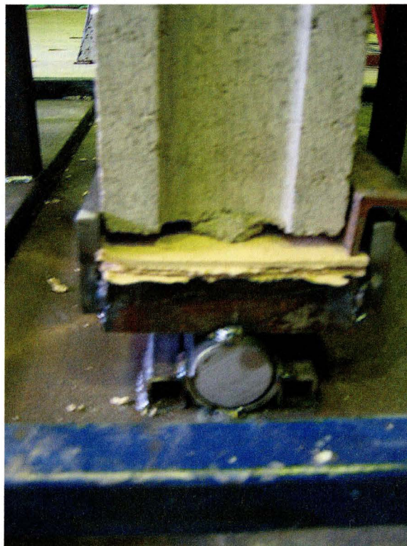
Figure 3.6 Pinned support configuration
