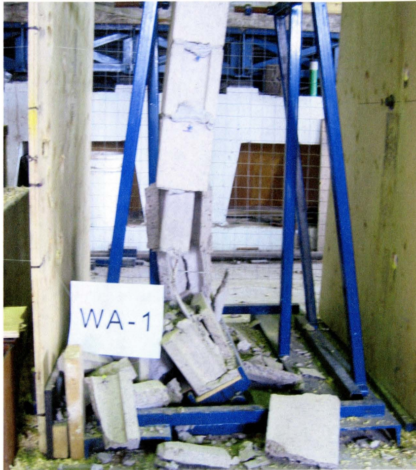
Figure 4.2 Failure mode of wall specimen WA-1
