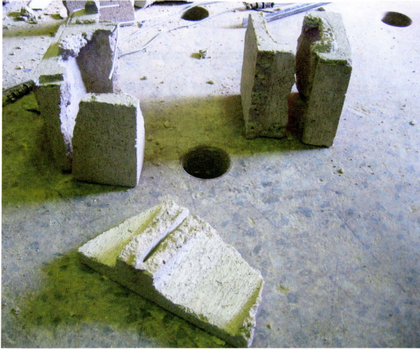
Figure 3.18 Web splitting in 3-high hollow prism test
