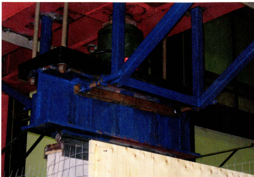
Figure 3.7 Loading arrangement and top bracing for wall test
