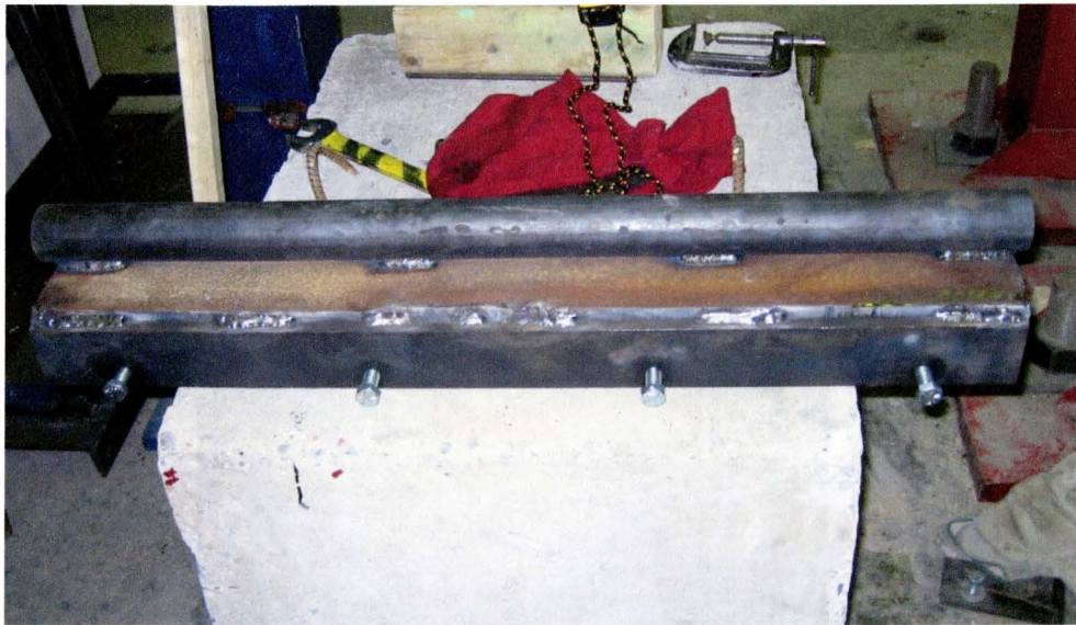
Figure 3.5 Close-up view of roller support
