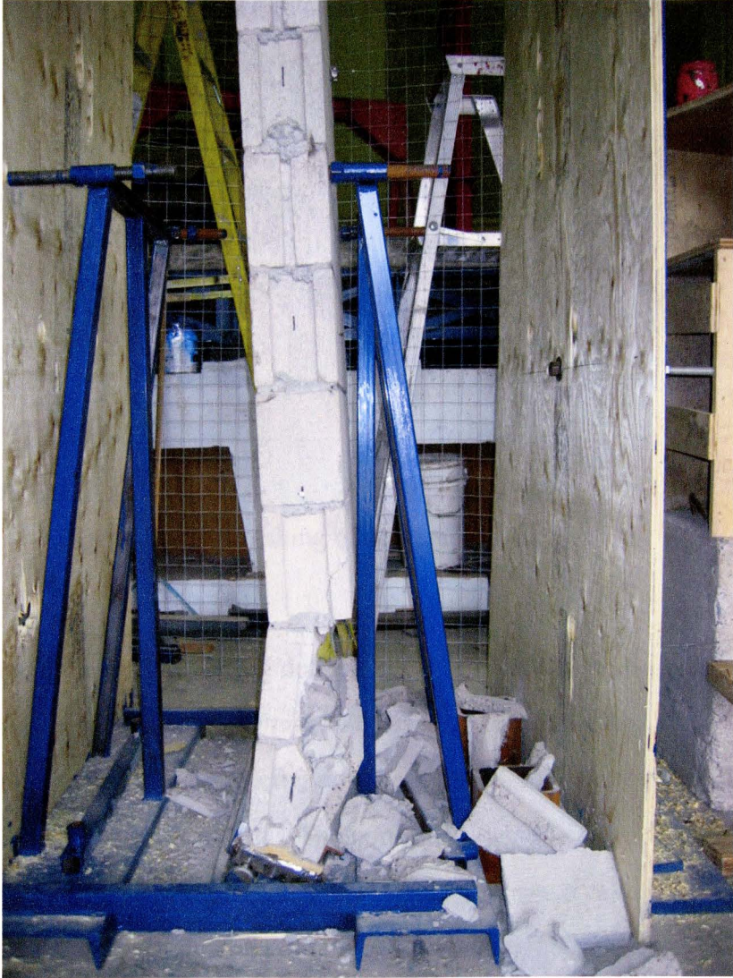
Figure 4.16 Failure mode of wall specimen WC-3
