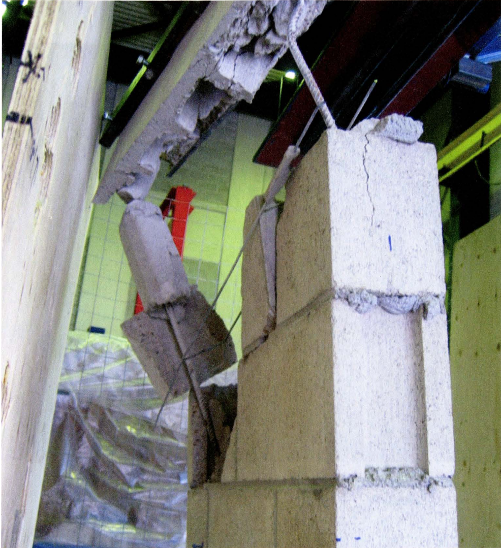
Figure 4.10 Failure mode of wall specimen WB-1
