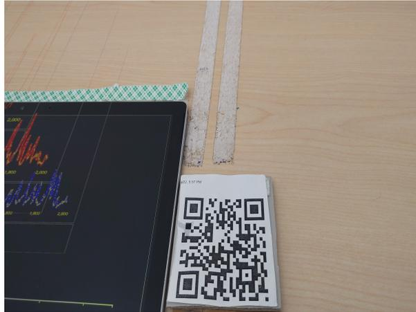
Figure 3.8: QR code attached to the tablet to align the AR contents
