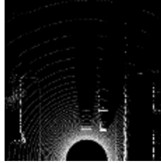
Figure 24 BEV image from LiDAR with 256 \times 256 pixels
