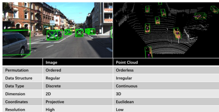
Figure 15 a comparison between image data and point cloud data [27]
