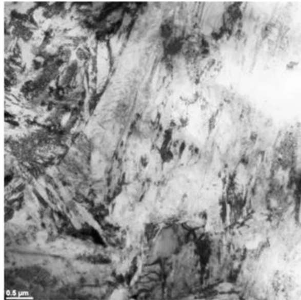
Figure 2.14: Micrograph of lath martensite in D2 at cooling rate of 50 K/s [57].
