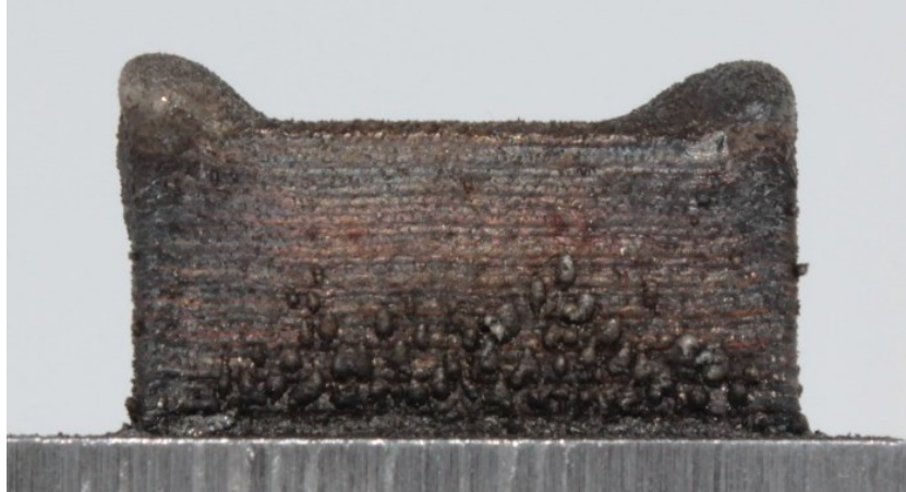
Figure 4.10: Sample D4, highlighting the more extreme ‘built-up’ corner effect, due to the scanning strategy employed (the cut substrate is shown at the bottom of the image).
