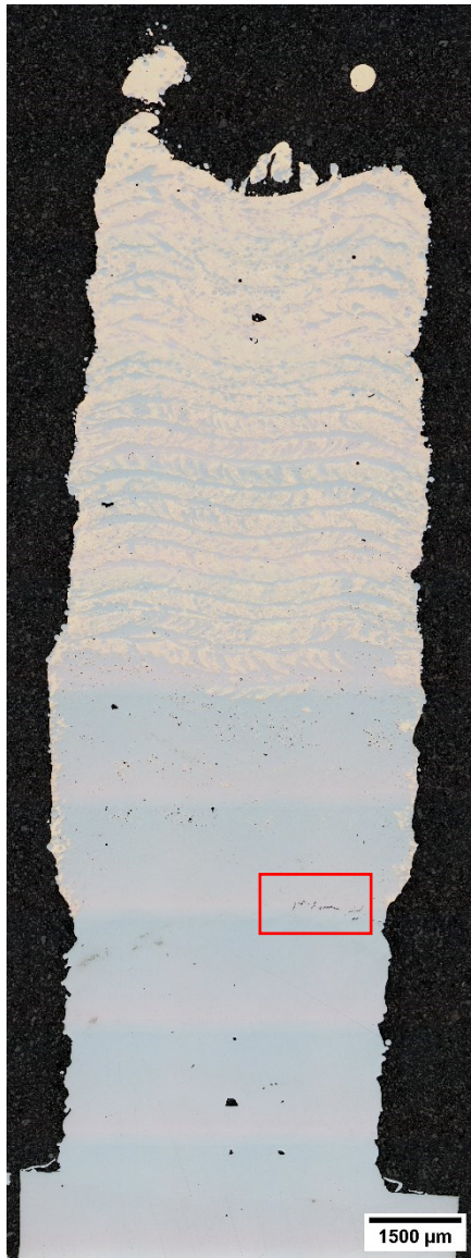
Figure 5.21: An H13-Cu FGM sample processed at 460 W with the solid red box indicating cracking, imaged using CLSM.
