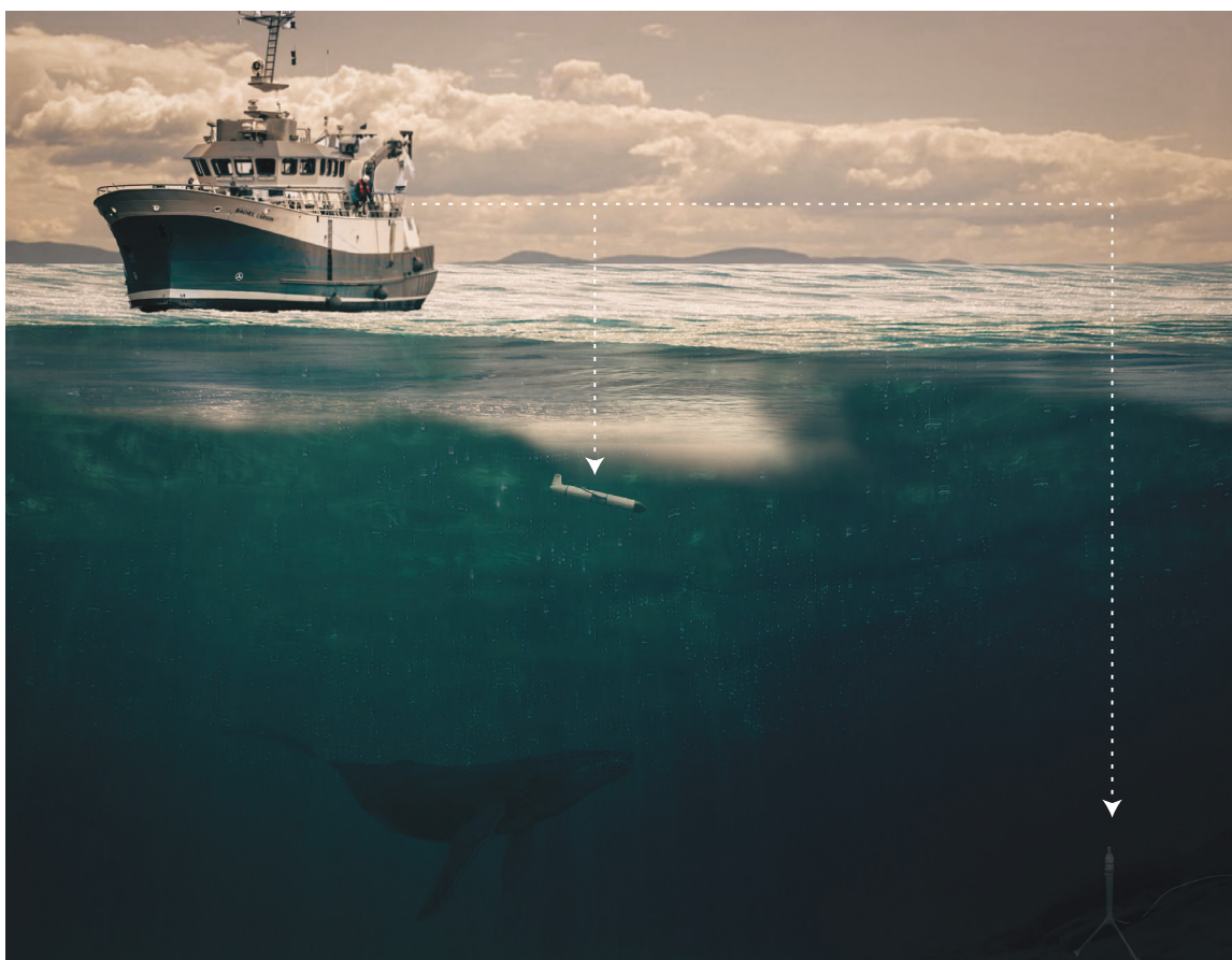
On and Below: The researcher uses recording devices like gliders and bottom mounted hydrophones to perceive below the surface, and translates these audio recordings for human perception. This demonstrates an invaluable ability to connect those above and below the surface through acoustic experiences.
