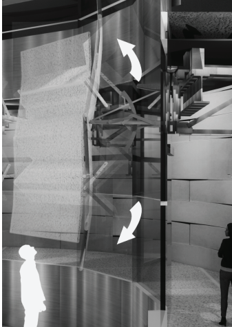
Detail view of operable dampener surrounding the 'Bay' room.
