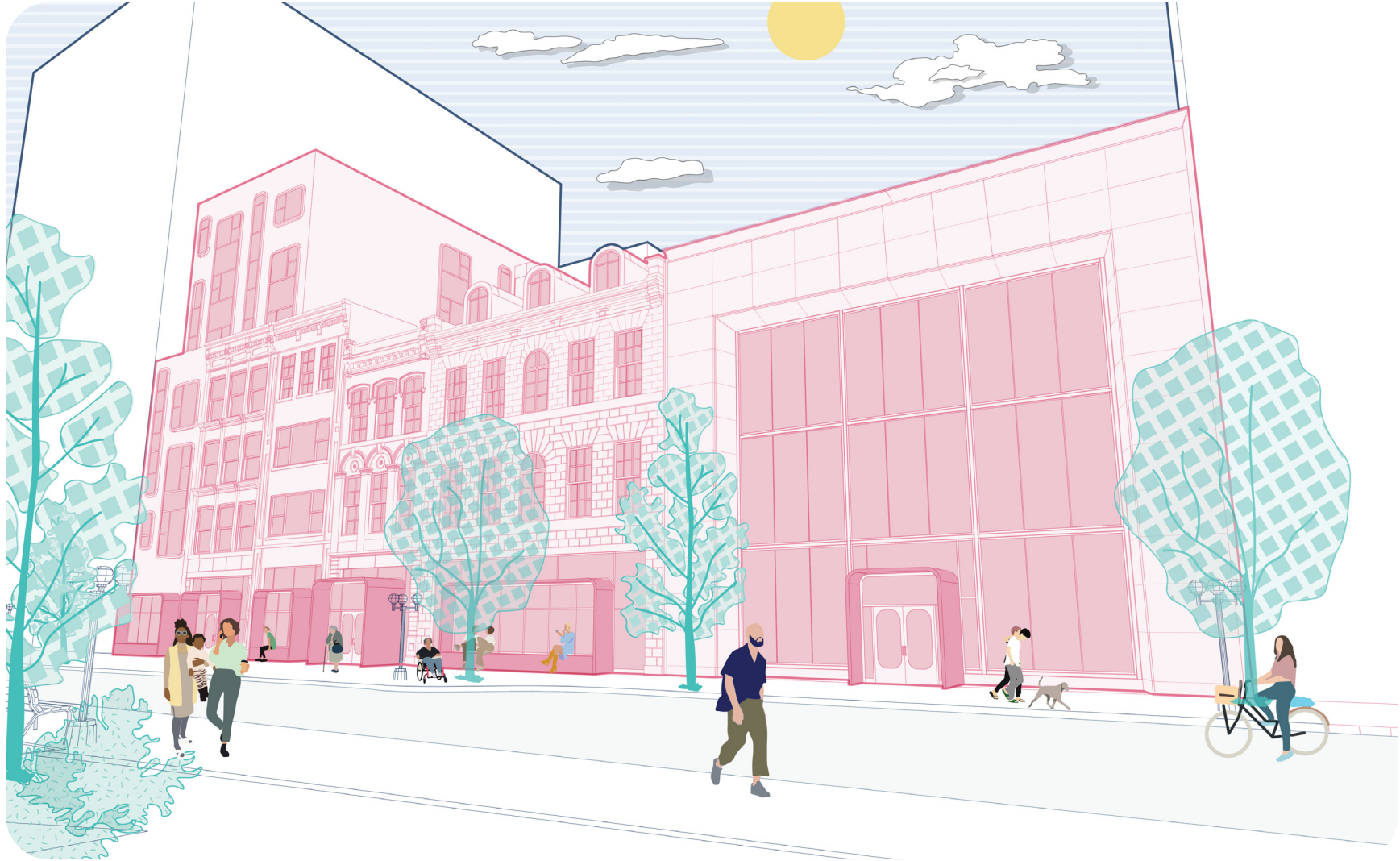
Exterior view of the front facade of Horizon House. Volumes are inserted through the existing glass openings on the ground floor to disrupt the flat boundary between inside and outside. The new addition to the building (on the left) both blends in and twists the order of the existing facade.
