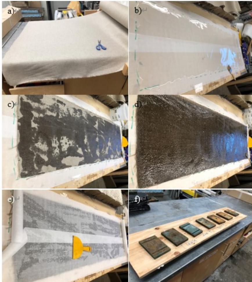
Figure 3-12 Sandwich panel fabrication: a) cutting flax fabric; b) applying a layer of resin; c) placing a layer of flax fabric; d) saturating flax fabric; e) removal of extra resin and air bubbles; f) placing core and weighed wooden board
