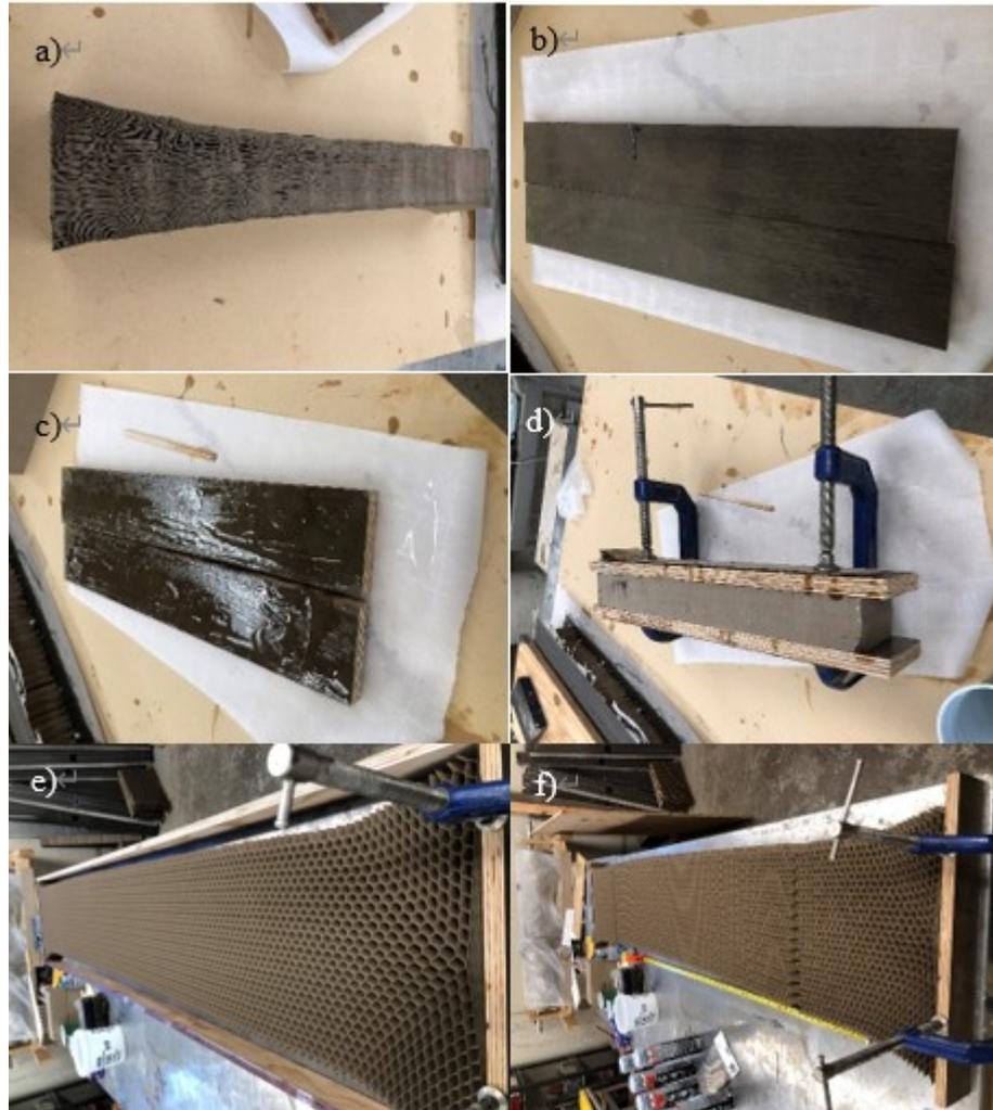
Figure 3-5 Core fabrication: a) unexpanded paper honeycomb; b) two wooden boards; c) applying epoxy resin to wood surfaces; d) curing with clips; e) stretching and setting; f) cutting
