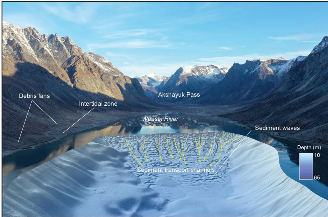
Figure 2.5: Composite image of multibeam bathymetry overlain on a UAV photograph of the fiord-head Weasel River delta. Debris fans extending to the intertidal zone, sediment waves and sediment channels are identified.
