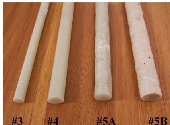
Figure 10. GFRP bars used for creep-rupture tests by Esmaeili et al. (2021).
