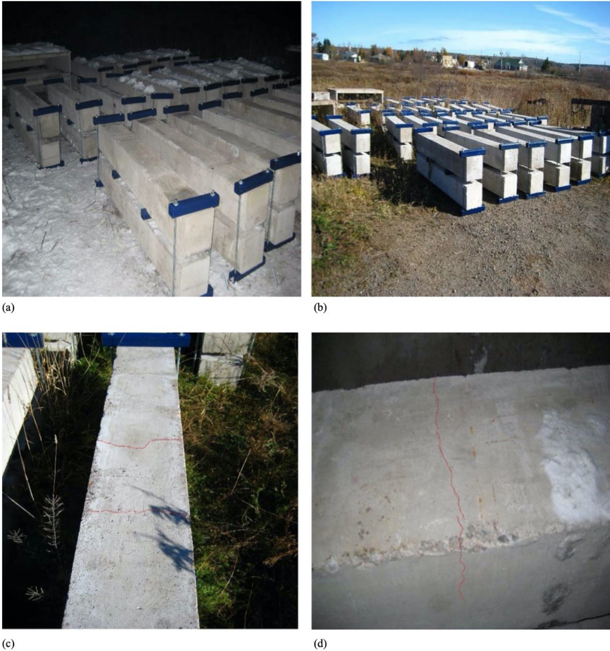
Figure 9. Photos of beams tested by Esmaeili et al. (2020): (a) beams under the sustained load and natural weather conditioning (December 2008); (b) beams under the sustained load and natural weather conditioning (October 2009); (c) number of cracks formed along the length of a conditioned beam; and (d) a close-up photo of a crack. (Images by John Newhook).
