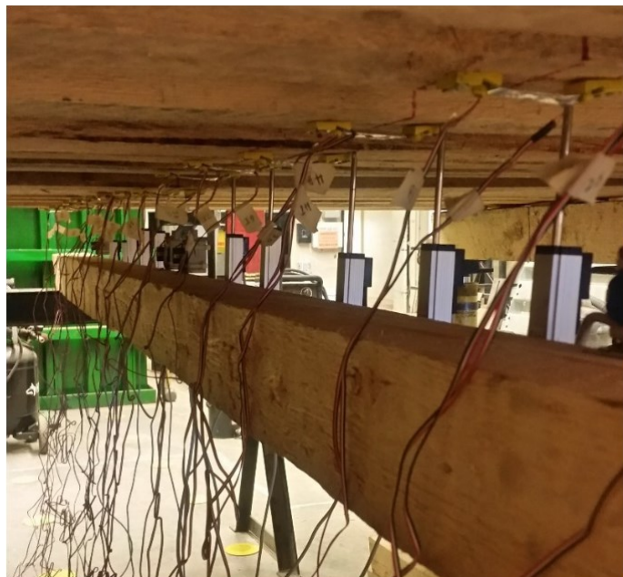
Fig. 2.7. Instrumentation of third scale bridge model (Smith 2018)
