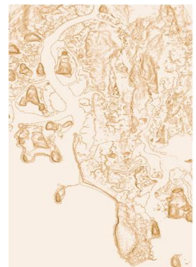
Figure 4 Slope raster of Pinkney's point, Nova Scotia created from DEM
