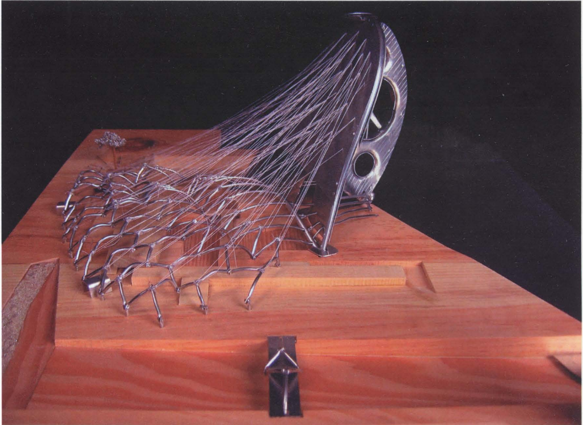
1 : 500 Structural model north facade of building
