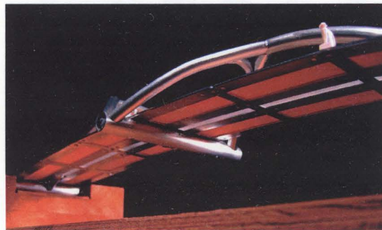
1 : 100 Bridge model showing structural glass
