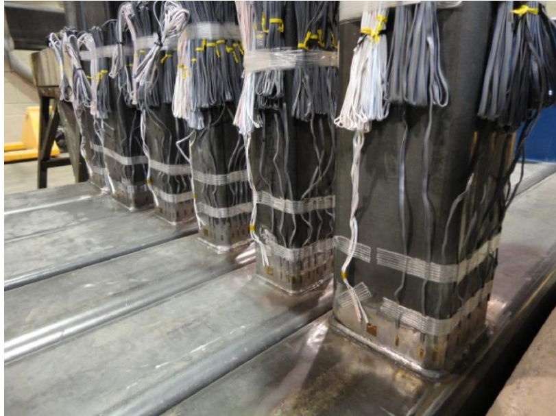
254 Fig. 9. Strain gauges adjacent to the welded joint for determination of uneven strain distribution in the 255 branch longitudinal direction [13] 256
