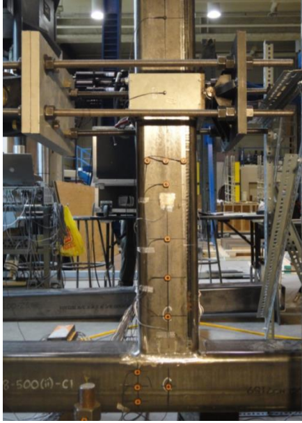
Fig. 3. Typical LED target locations [13]
