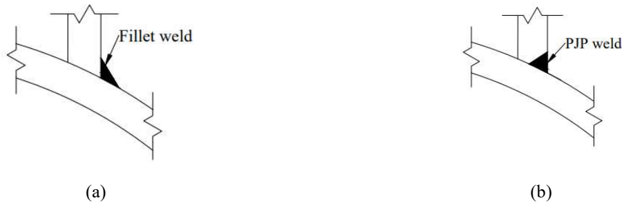
Figure 3-1 CHS-to-CHS moment T-connection weld configurations: (a) fillet weld and (b) PJP weld
