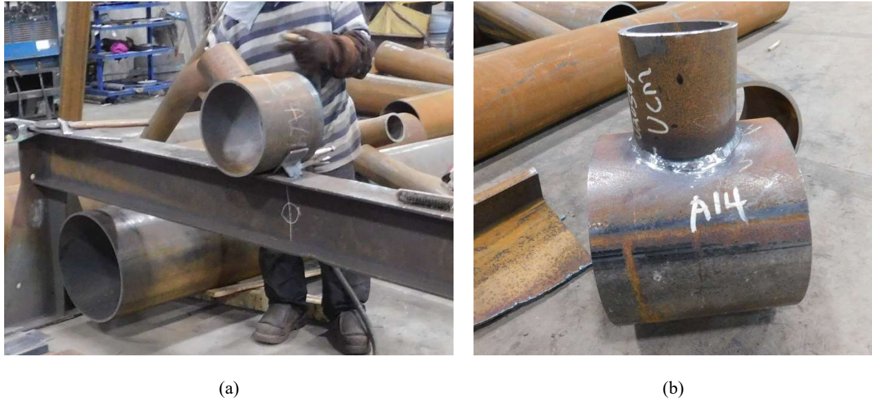
Figure 3-3 Welding of trial specimens: (a) before welding (b) after welding
