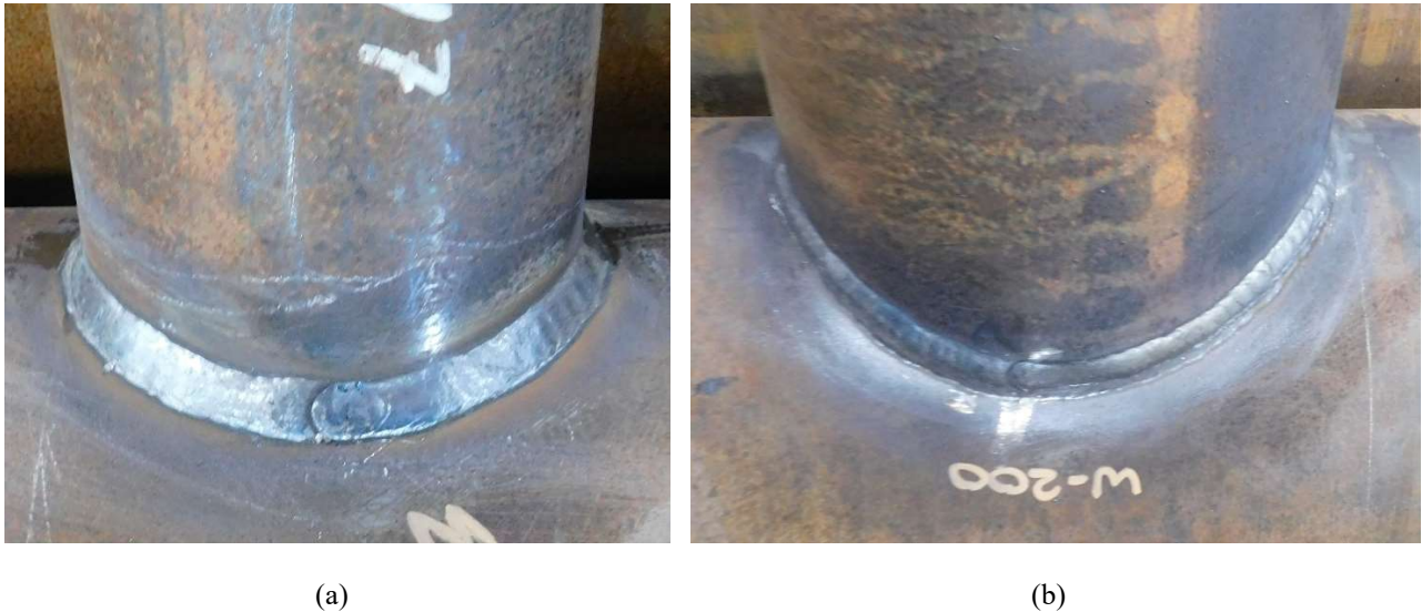
Figure 3-8 Final welded CHS-to-CHS T-connections: (a) fillet welds and (b) PJP welds
