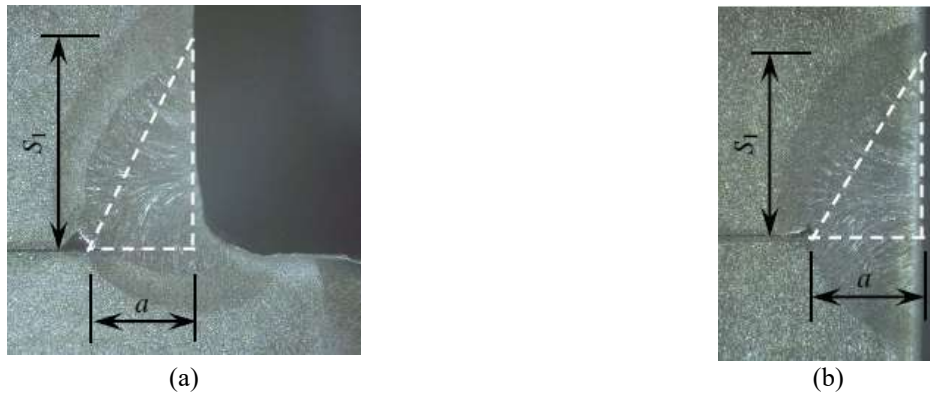
Figure 2-5 Typical macro etched specimens: (a) PJP-T joint and (b) PJP-B joint (Luo et al. 2020)
