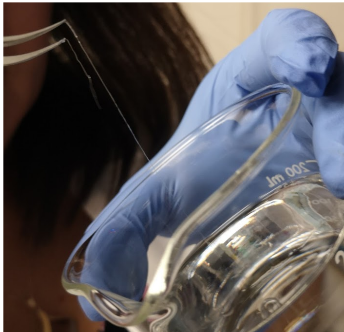
Fig. 3.11. Fibre of reduced W_2M being hand-drawn technique from ethanol bath.
