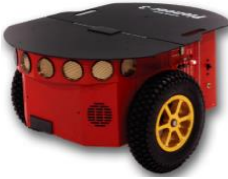
(a) Pioneer P3-DX ( 0.46 \times 0.38 \times 0.24 in meters)
