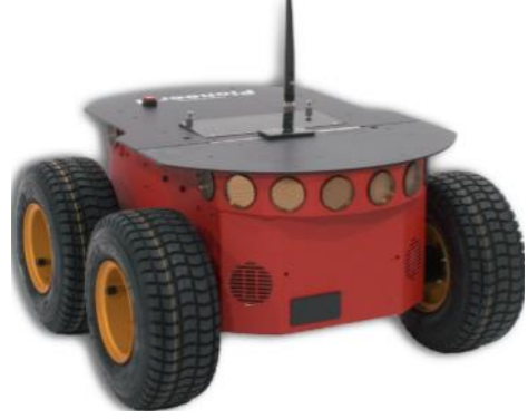
(b) Pioneer P3-AT ( 0.51 \times 0.50 \times 0.28 in meters)
