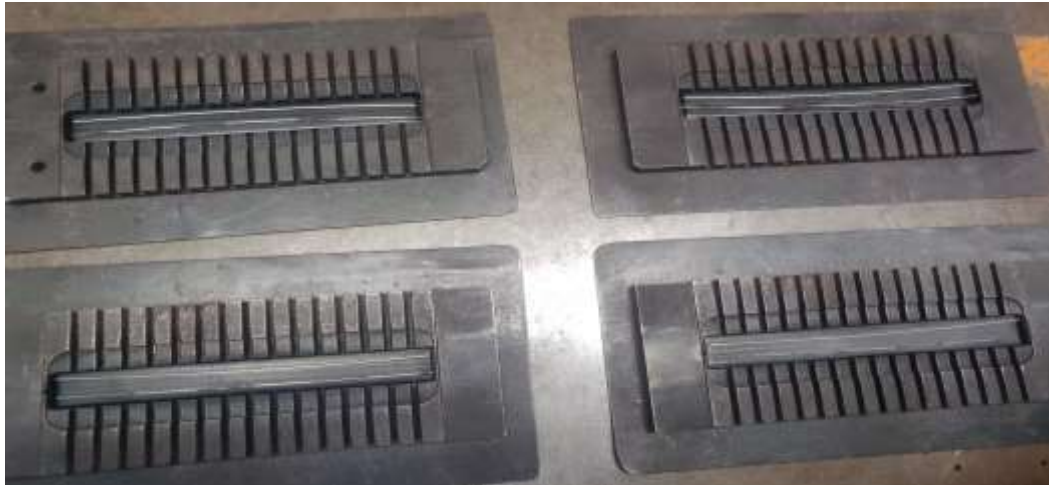
Figure 43: Lower side strip of green rubber inside the jig mold before curing.
