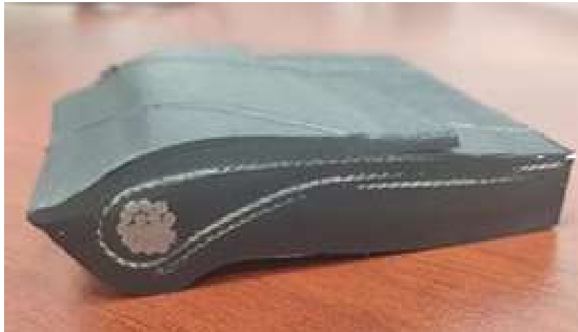
Figure 12: Cross sectional area of tire bead
