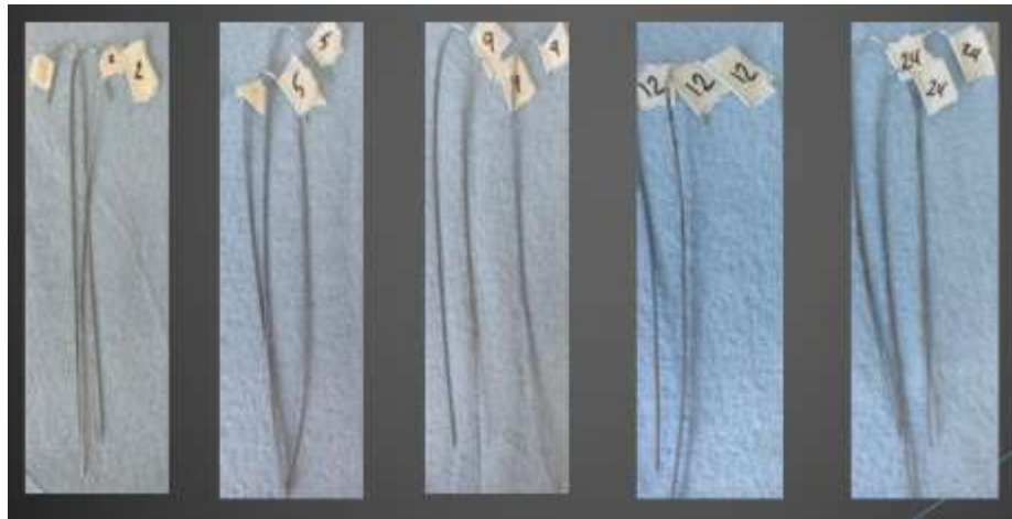
Figure 39: Tringle wires dipped in water for various period.
