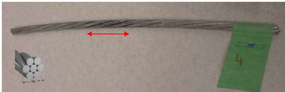
Figure 62: 2m of corroded circumference of bead wire
