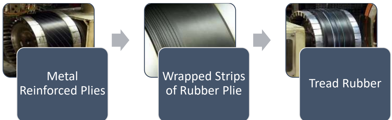
Figure 4: Tread section manufacturing process
