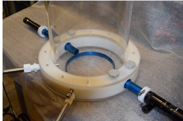
Figure 4.2 The inter-flange spacers (provided with ports to hold a wide variety of instruments at 4 locations along with the height of the contactor).
