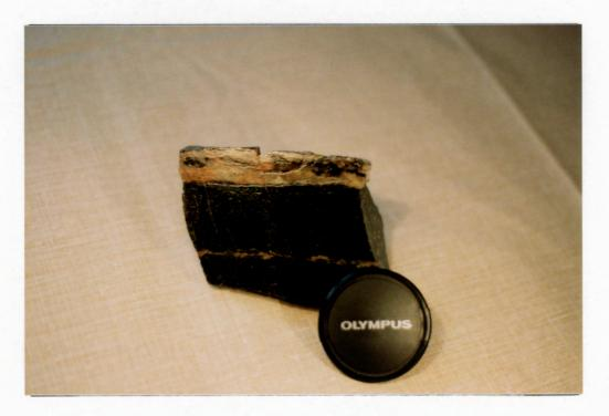
Figure 2.25. Amphibolite gneiss with gneissic banding.
