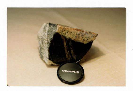
Figure 2.27. Biotite-quartz-feldspar xenolith in a granitoid dyke. The xenolith still contains the pervasive foliation and gneissic segregation.
