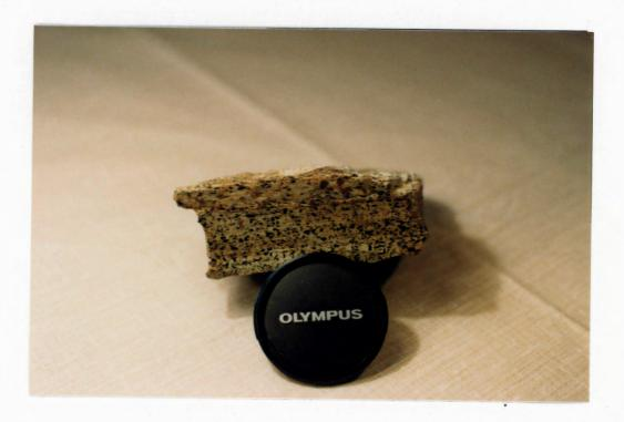
Figure 2.11. Porphyroblastic staurolite, garnet and biotite in the phyllite of Metasedimentary Unit 2.
