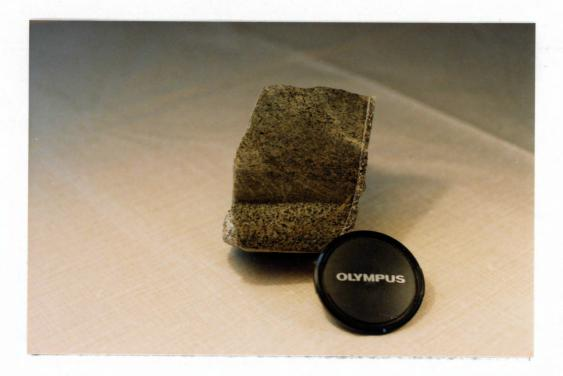
Figure 2.7. Compositional banding parallel to the foliation in the phyllite of Metasedimentary Unit 2.
