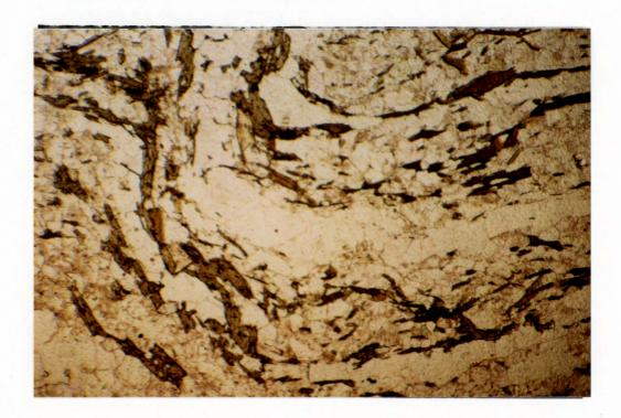
Figure 3.16. Crenulations of the fabric defined by the parallel alignment of biotite, chlorite and epidote in the Jumping Brook Granitoid (plane polarized light, x 31.25).
