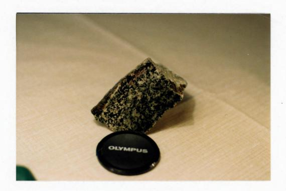
Figure 2.18. Diorite near to French Lake showing coarse grained nature, no fabric and purple mineral (possibly fluorite) near the top of the sample.
