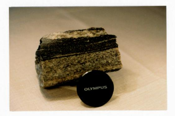
Figure 2.23. Biotite-Quartz-Feldspar gneiss (a) with garnets (b) with gneissic segregation.
