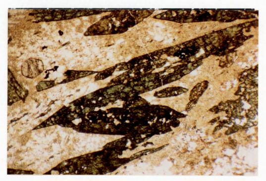
Figure 3.11. Idioblastic, poikiloblastic, hornblende porphyroblasts within the psammite of Unit 2. (crossed polars, x 31.25).
