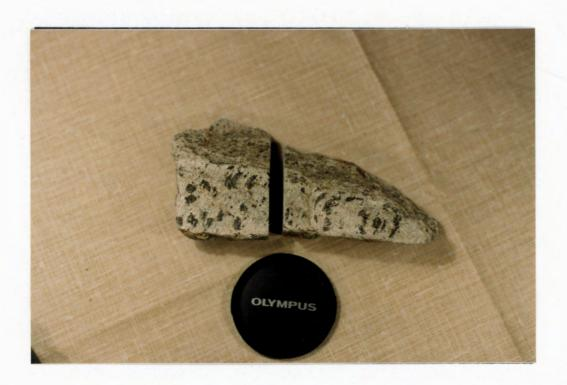
Figure 2.9. Porphyroblastic biotite within the phyllite of Metasedimentary Unit 2.
