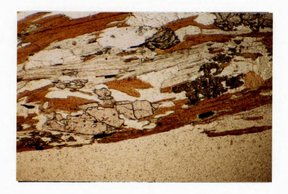
Figure 3.13. Pre-tectonic kyanite in the biotite-quartz-feldspar gneiss, fractured and elongated parallel to the schistosity. (plane polarized light,  $\times$  31.25).
