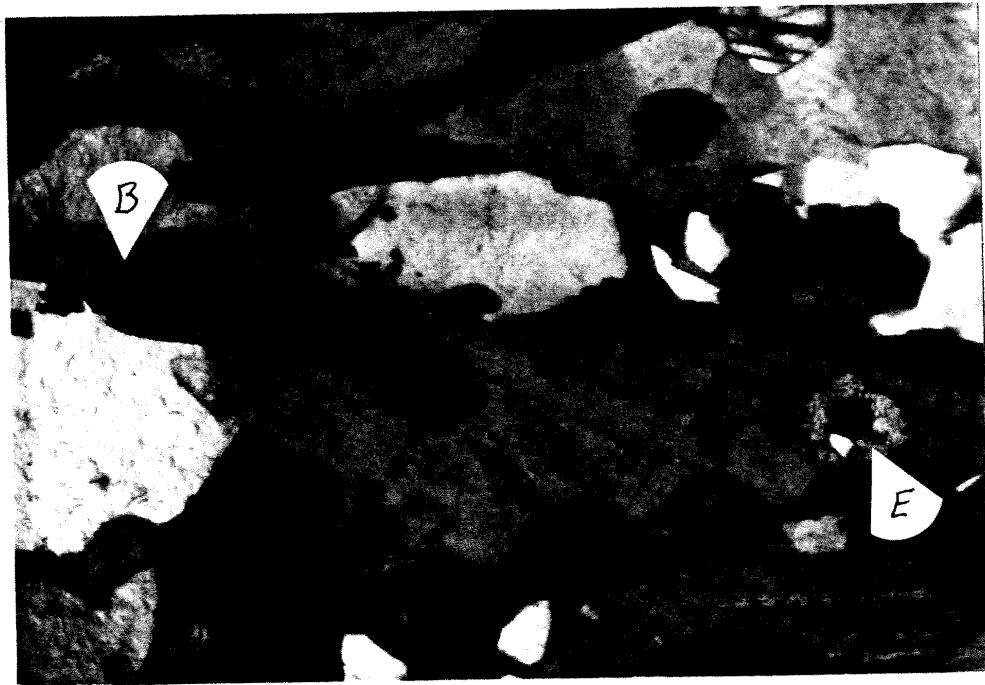
Photo 3.20 Gneiss showing elongate biotite (B) and idioblastic epidote with allanite core (E) in quartz-feldspar matrix (KJ13). (XN).
