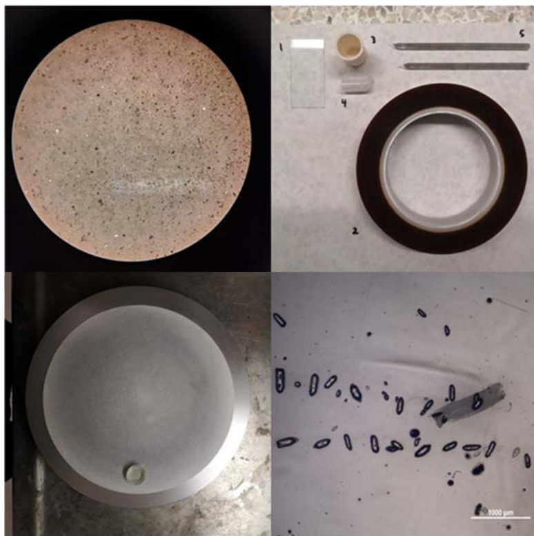
Figure 6 (a) Entire field of view of original pan concentrate from which individual zircons are selected. (b) Utensils used to pick zircon crystals: (1) thin section slide, (2) double sided tape, (3) alumina container for (4) silica crucible, and (5) silica rods with melted ends to pick crystals. (c) 0.3 µm disc for polishing epoxy puck (sitting on disc). (d) Polished puck with sample 18JC0008 zircon under transmitted light microscope.
