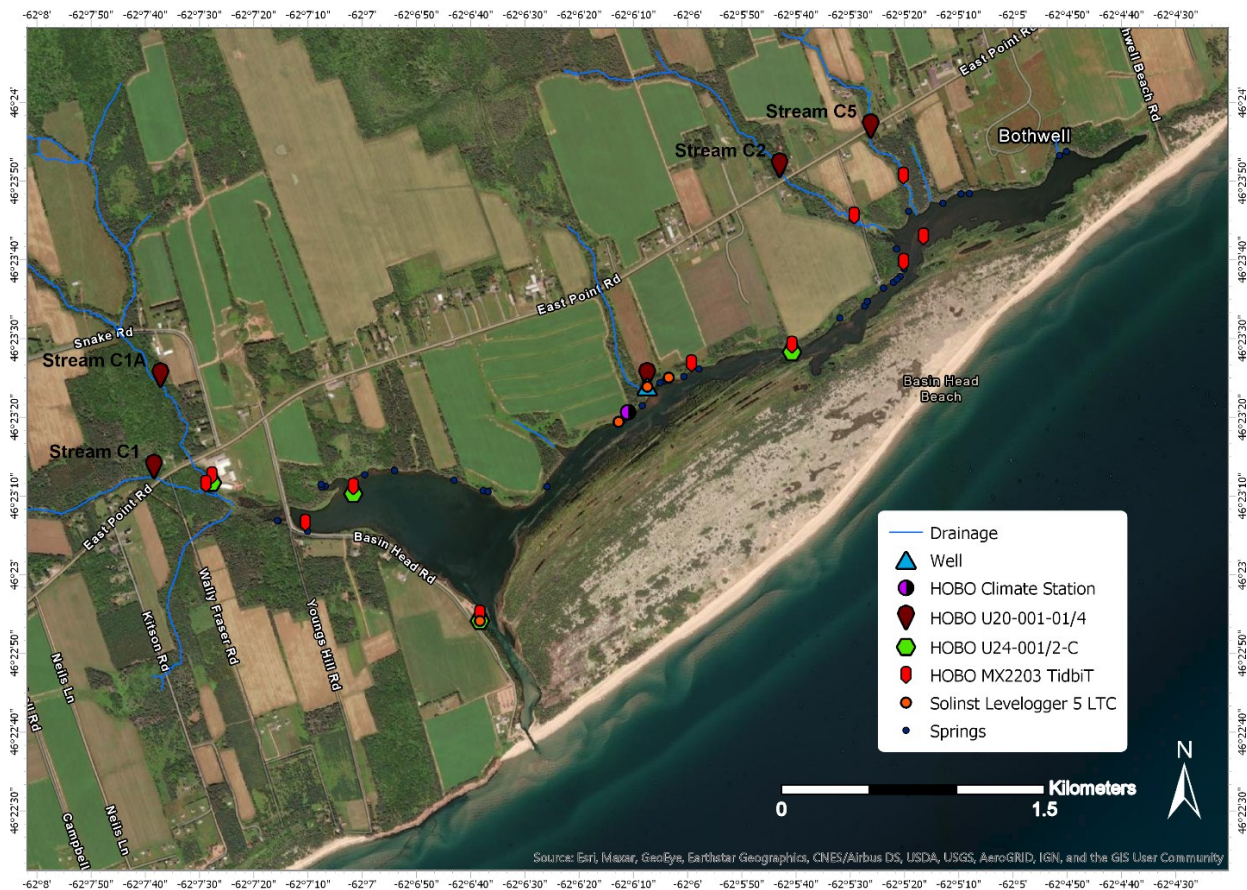
Figure 7. Map outlining the locations of temperature loggers (Onset HOBOb® MX2203 TidbiT), conductivity loggers (Onset HOBOb® U24-001/2-C), pressure transducers (Onset HOBOb® U20-001-01/04), pressure-temperature-conductivity loggers (Solinst Levellogger 5 LTC), the Dalhousie piezometer (Well), and Onset HOBOb® weather station within the Kingsboro watershed for their respective sampling periods during 2019-2020. Sensors with short-term deployments (<2 weeks) were not included in this figure. Near-shore springs and stream locations are indicated. Map prepared in ArcGIS Pro (Version 2.3.3, 2018).
