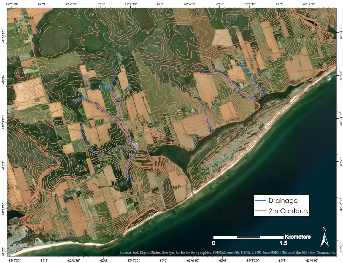
Figure 32. Topography and drainage patterns of the Kingsboro watershed. The area is generally gently sloping (2-5% slopes), with the steepest portions being located along the shore. The maximum elevation is approximately 60 metres. Topography data was sourced from the PEI Dept. Env. (2008). Map prepared in ArcGIS Pro (Version 2.3.3, 2018).
