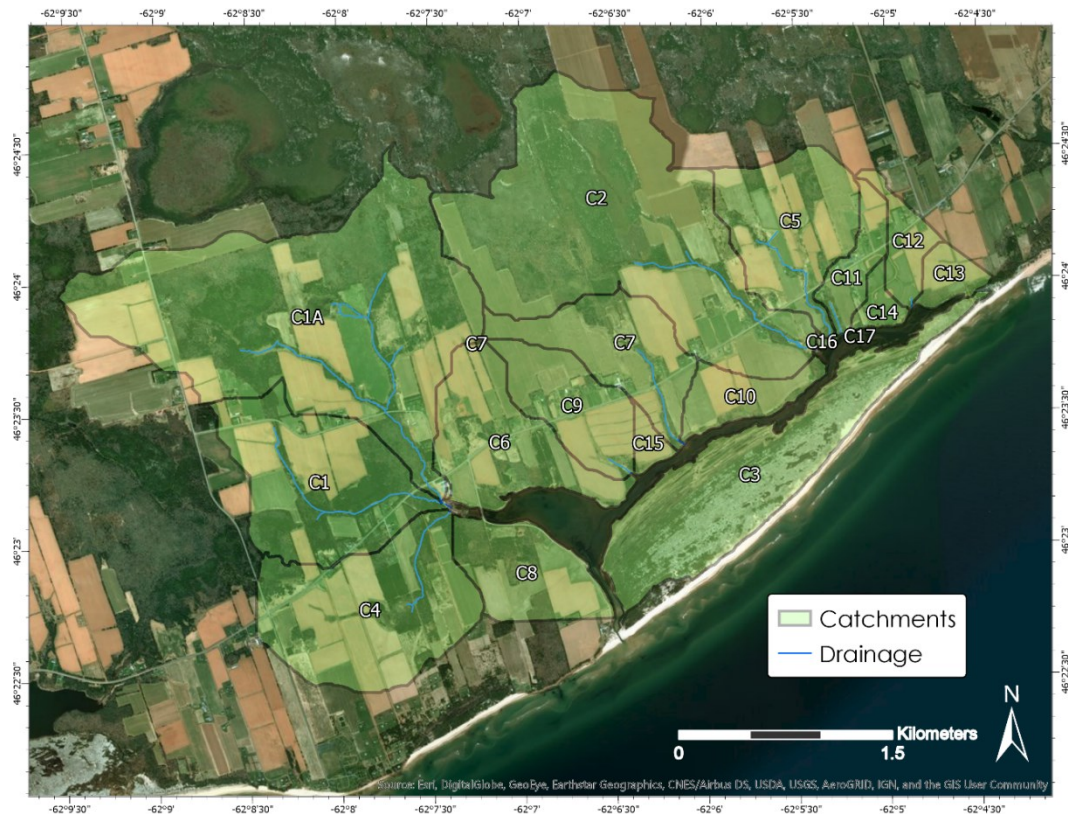
Figure 2. Topographically determined subcatchments of the KW watershed and their associated drainage networks. The total KW area is approximately 14.6 km 2 , and each catchment is denoted by C1-C17, for a total of 18 subcatchments. Streams are designated by their respective subcatchments (e.g., Stream C1A). The major western streams (i.e., Streams C1, C1A, and C4) all converge in an intertidal salt marsh to form the largest stream discharge into Basin Head Harbour. Map prepared in ArcGIS Pro (Version 2.3.3, 2018).
