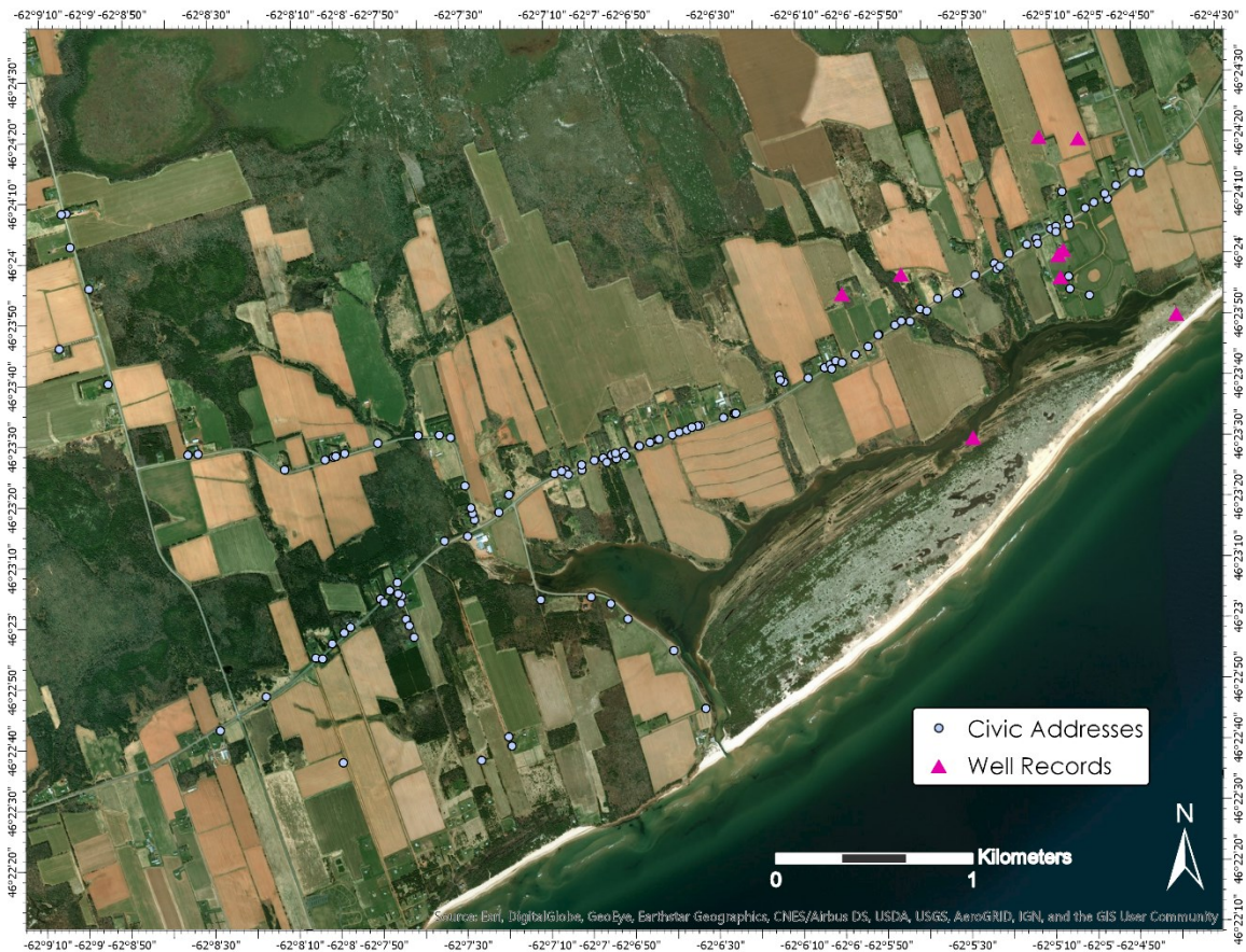
Figure 36. Well logs within the Kingsboro watershed that the provincial authority has on record (i.e., 9 pink triangles), as well as the record of civic addresses in the area (i.e., 127 blue circles). This map, coupled with the most recent land use inventory displayed in Figure 35, suggest that several wells are unaccounted for. Map prepared in ArcGIS Pro (Version 2.3.3, 2018).
