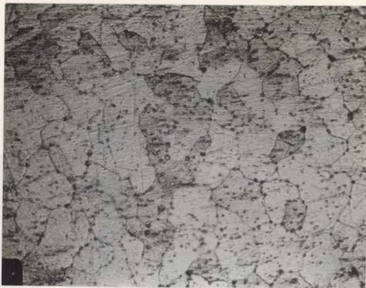
Fig. 10a Microstructure of Silmanal quenched and etched with \text{CrO}_3\text{-H}_2\text{SO}_4 . (x 500)
