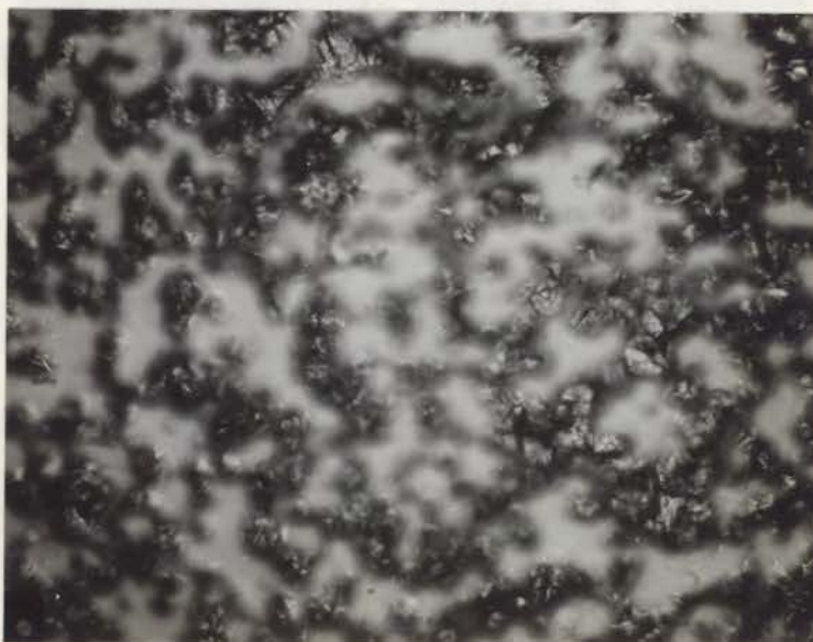
Fig. 16 b Micrograph taken in polarized light from \text{Ag}_{0.1}\text{Mn}_{1.11}\text{Al}_{0.89} aged at 300^{\circ}\text{C} and etched with \text{HNO}_3\text{-HCl} . (x 800). The microstructure indicates three phases, the hard phase in "Maltese Cross" pattern.
