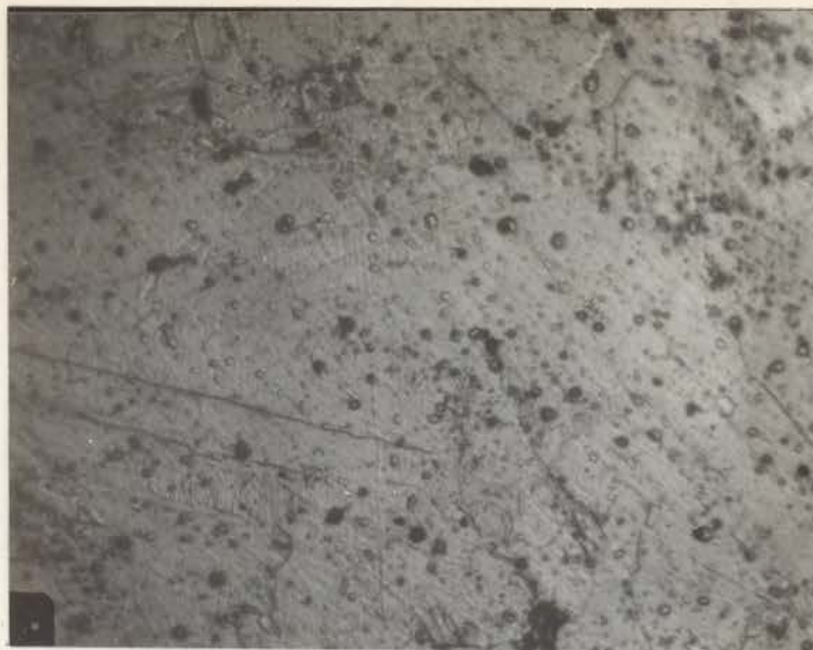
Fig. 16a Micrograph of \text{Mn}_{1.11}\text{Al}_{0.89} aged at 300^{\circ}\text{C} and etched with \text{HNO}_3\text{-HCl} acid. (x 500). The structure indicates two phases.
