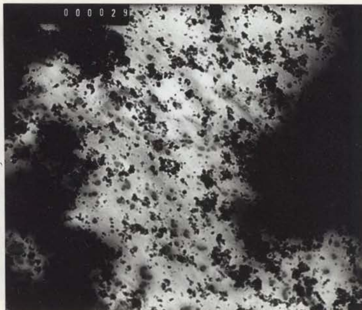
Fig. 16 d Electron transmission micrograph taken from a magnetic colloid replica of \text{Ag}_{0.2}\text{Mn}_{1.11}\text{Al}_{0.89} aged at 300^{\circ}\text{C} . (x 14840). The replica indicates the fairly homogeneous distribution of magnetic particles in clusters grown to different sizes.
