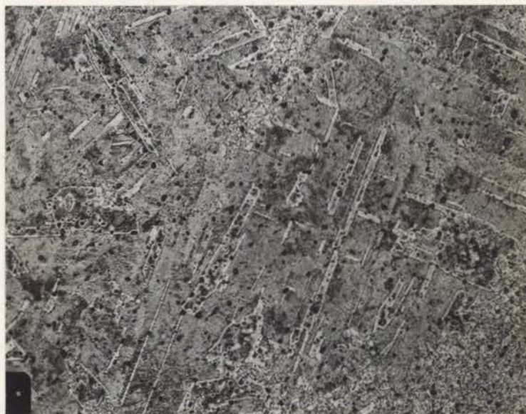
Fig. 10e Microstructure of Silmanal aged at 400°C for 168 hours, etched with \text{CrO}_3\text{-H}_2\text{SO}_4 . Typical Widmanstätten structure (x 500)
