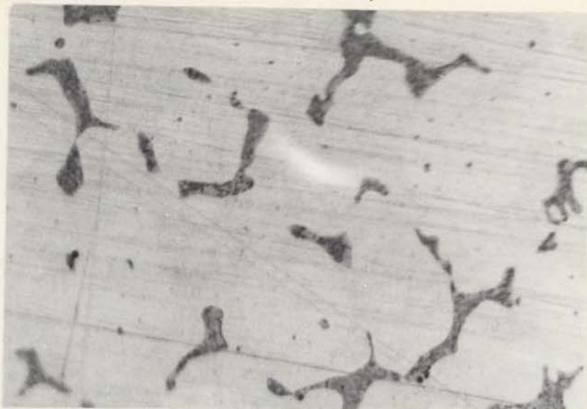
Fig. 20a Micrograph of Ag_5MnSb alloy aged for 200 hours unetched. (x 500)
