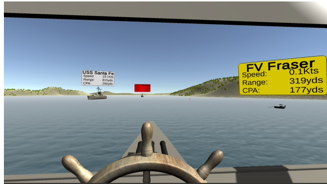
Figure 7.9: The Ship Avoidance ARNA provides a textual overlay in position with other vessels. The text is displayed upon a panel that remains oriented towards the observer. The text informs the NavO of the name of the vessel, current range, and CPA.
