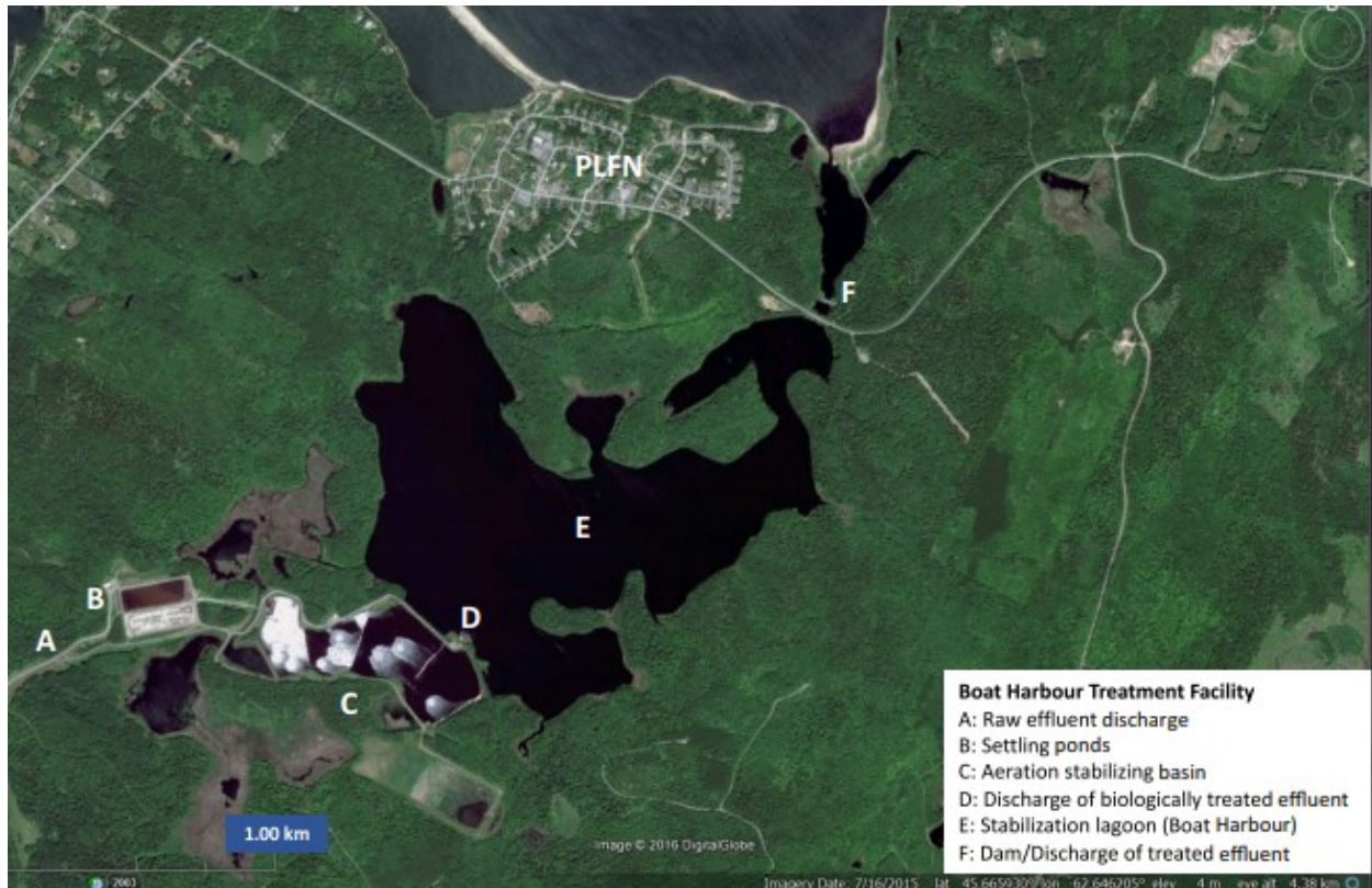
Figure 6. Map of Boat Harbour Effluent Treatment Facility (BHETF) and its surrounding area (Hoffman et al. , 2017). Pictou Landings First Nation (PLFN), whose physical proximity and loss of traditional use of the Boat Harbour former tidal estuary are of primary concern to issues of water treatment, lies between the Northumberland Strait and the BHETF.
