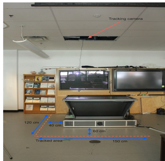
FIGURE 2: SETUP OF PROXIMITYTABLE, KINECT CAMERA INSTALLED IN THE CEILING FOR TOP-DOWN TRACKING, TWO SIDES AROUND THE TABLE ARE BEING TRACKED
