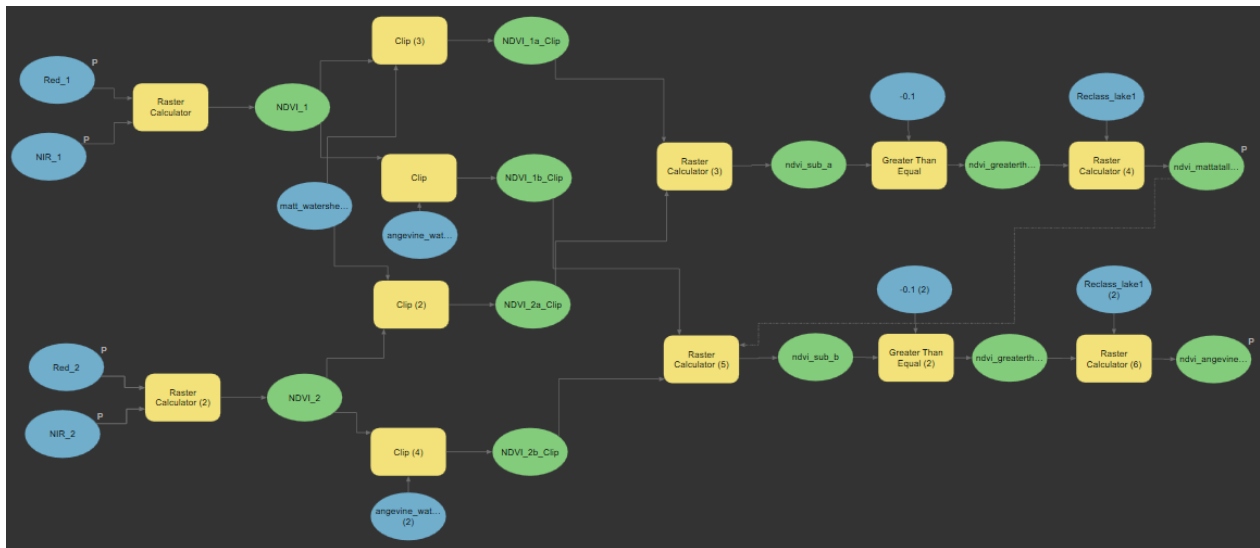
Figure A.3: Model used to subtract the NDVI raster layer values using the Greater Than Equal function on ArcGIS Pro (ESRI Inc., 2018).
