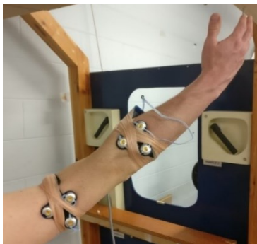
Figure 8 IREDs in triads attached to both arm and forearm of participant.
