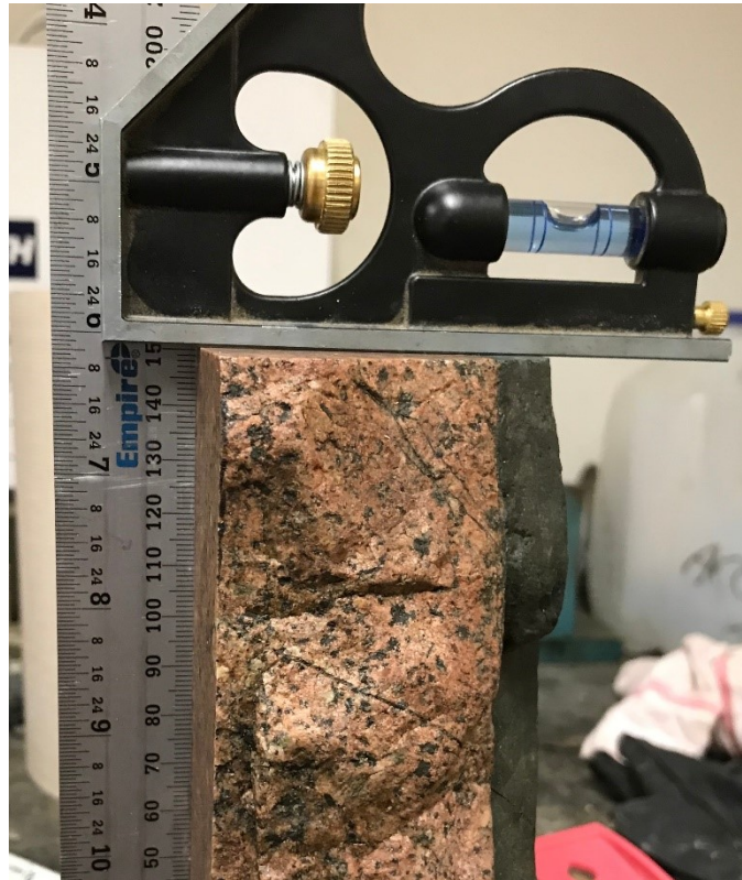
Figure 3-9: First vertical cut made perpendicular to the primary rock specimen bottom and secondary to primary rock contact line.
