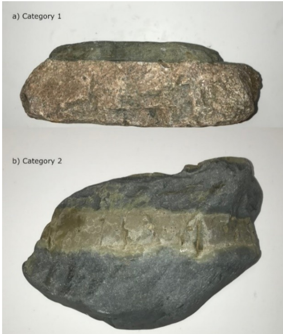
Figure 3-6: Example of boulders with two different procedures for block extraction: a) Category 1: blocks can only be taken from one side of the secondary rock; b) Category 2: blocks can be taken from both sides of the secondary rock.
