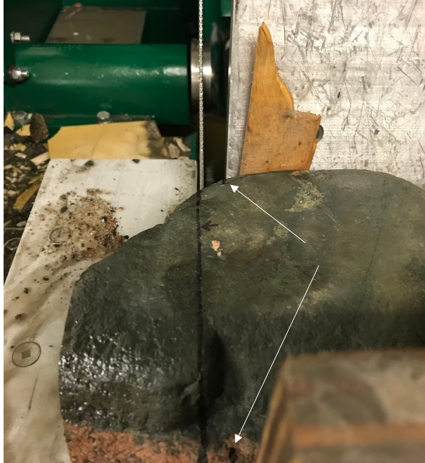
Figure 3-8: Cut line displaying arrow indicating the final dimension of the cut-off piece is to be taken to edge of the line indicated with a black arrow. Photo shows a boulder fastened in the cutting machine vise with the cut line aligned with the cutting wheel and the guide marks aligned with the edges of the upright vise components.
