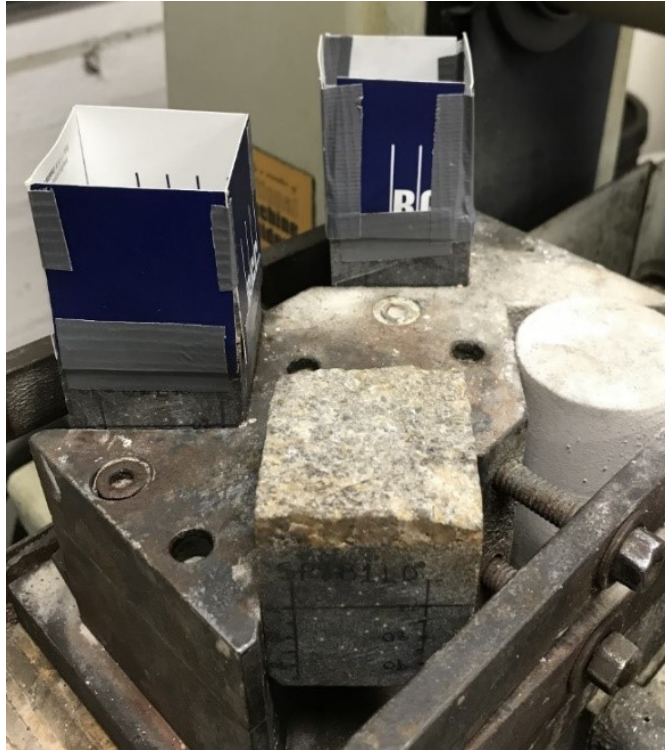
Figure 3-11: Three rock type transition block specimens aligned in the v-notch block on the grinder. On all specimens, the Leeb strikes can be seen on the visible face (method 1, Section 3.1.2.4) as well as the marked line aligned with the top of the v-notch block.
