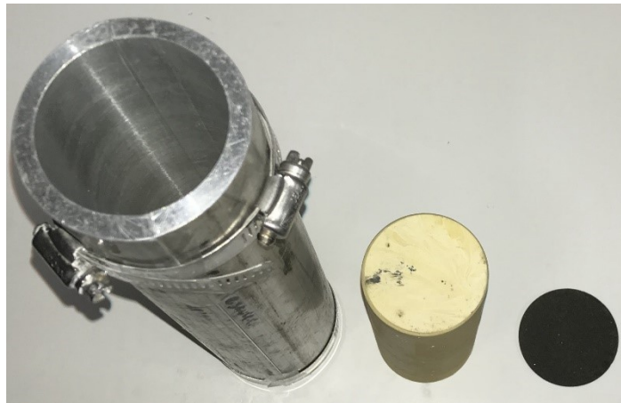
Figure 3-2: Objects used to create artificial material UCS specimens. From left to right: stainless steel dual specimen cast, cured artificial material specimen, and a thin sandstone disk.
