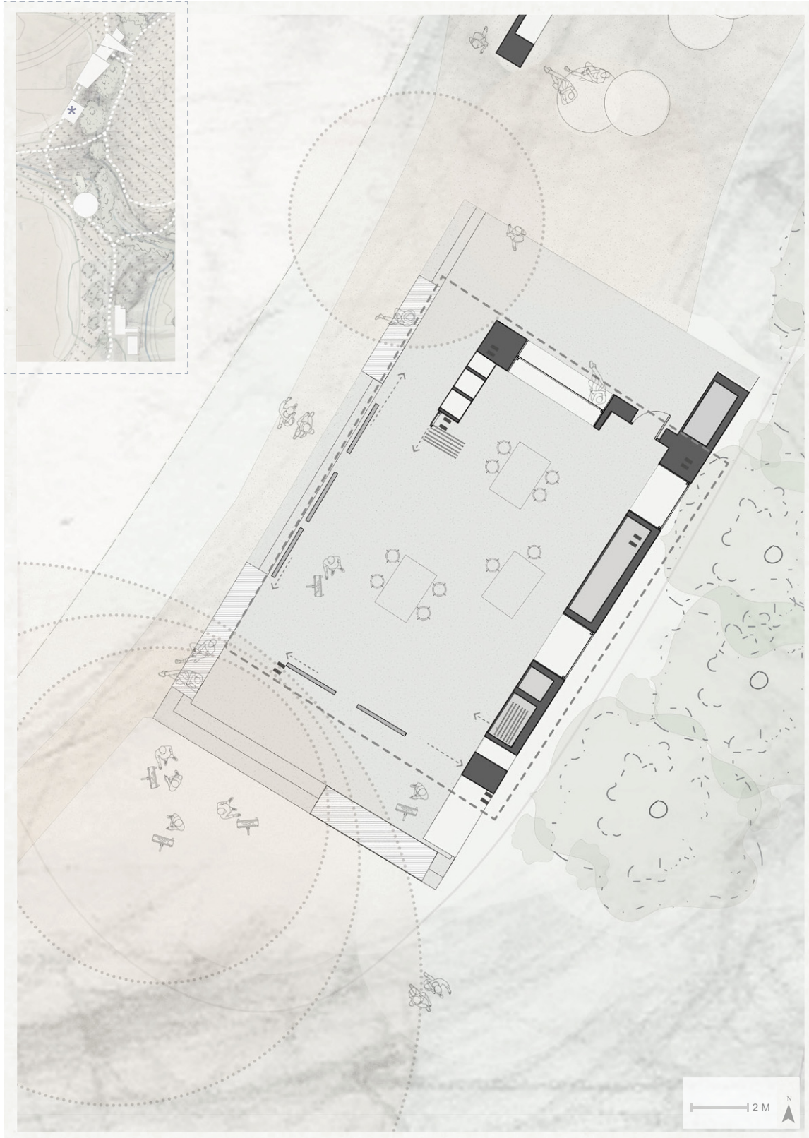
Inhabited plan showing workshop with flexible accordion curtain walls and shifting screens that enable workshop to transition into a continuous extension of the landscape and path. Image depicts examples of activated outdoor spaces hosting art classes and areas to sit, study, etc.
