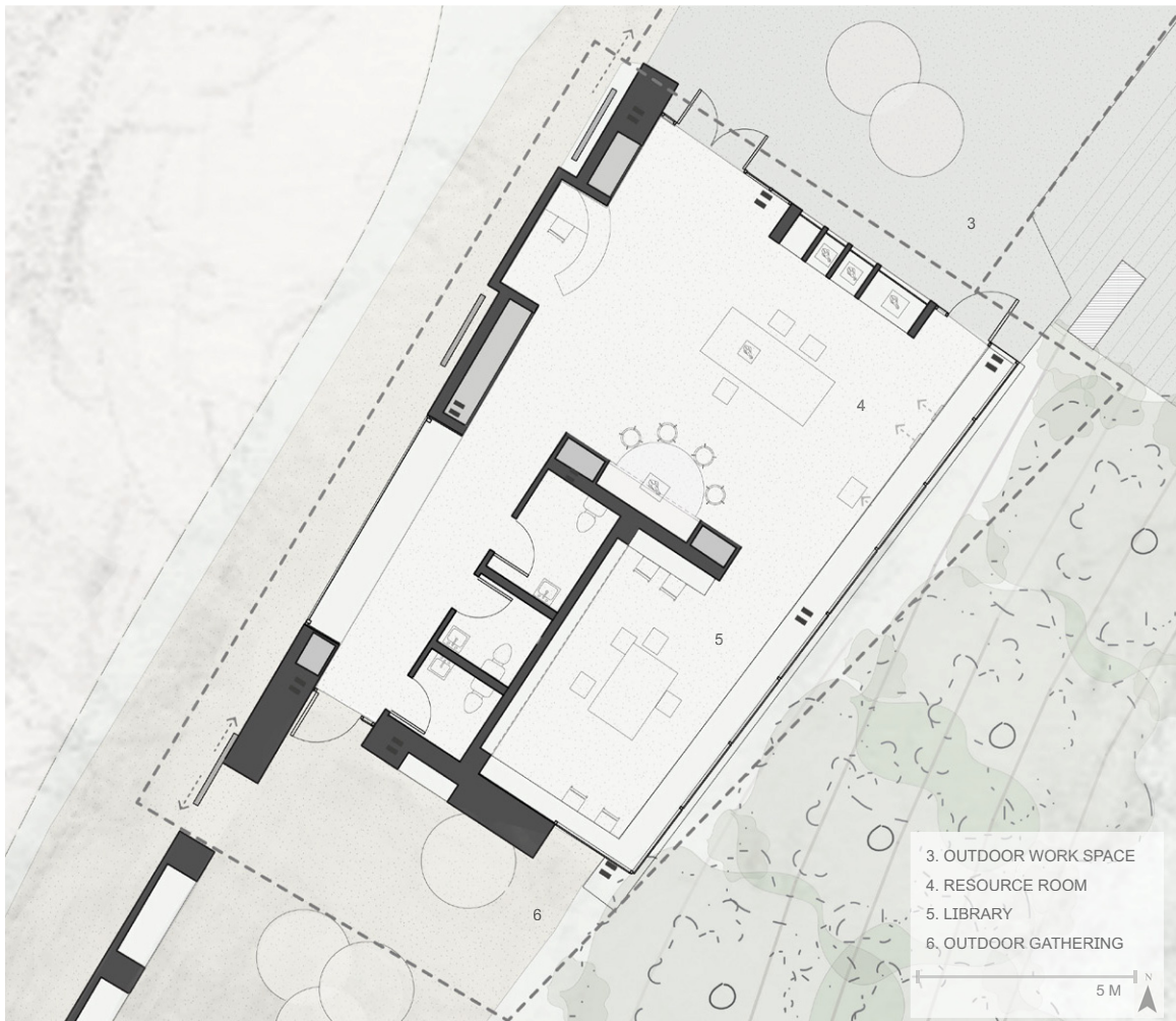
Top: Key plan locating interior resource spaces. Bottom: Plan showing interior resources spaces of the Resource Center.
