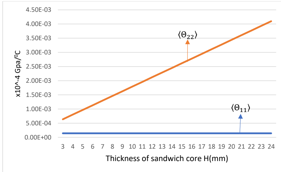
Figure 6.52 Thermal coefficients of a sandwich rib structure
