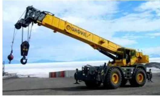
Figure 10: With mobile cranes, the operator is near ground level and safe from emissions.
