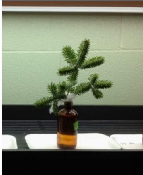
Figure 15. Experimental set up of balsam fir branch, wrapped with gauze, and placed in amber bottle.
